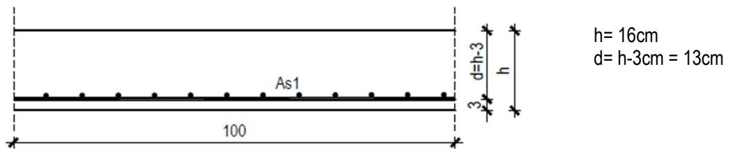
**Beton:** C 30/37  $f_{ck}=30.0 \text{ MPa} \rightarrow f_{cd} = \frac{f_{ck}}{\gamma_c} = \frac{30}{1.5} = 20.00 \text{ MPa}$
