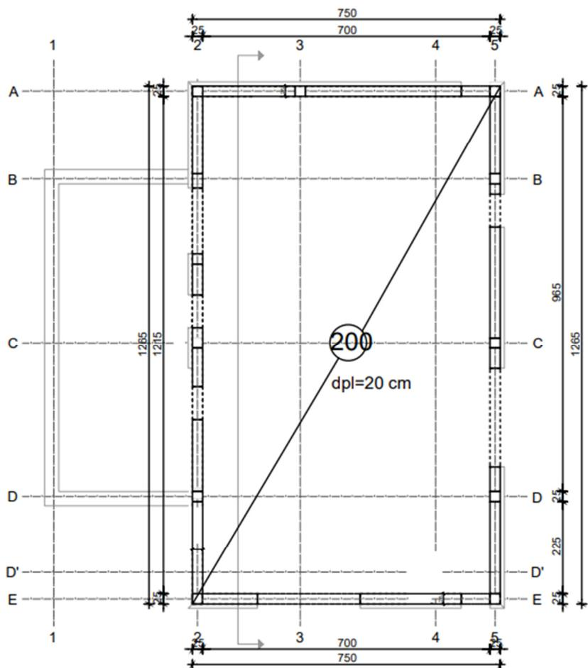
Beton: C 30/37;  $f_{ck}=30.0 \text{ MPa}$ ;  $f_{ctm} = 2.9$
