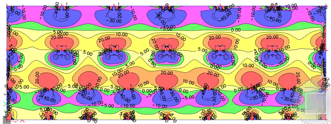
Slika 6.18 Poprečne sile  $V_{Ed,y}$  (kN/m) za GSN
