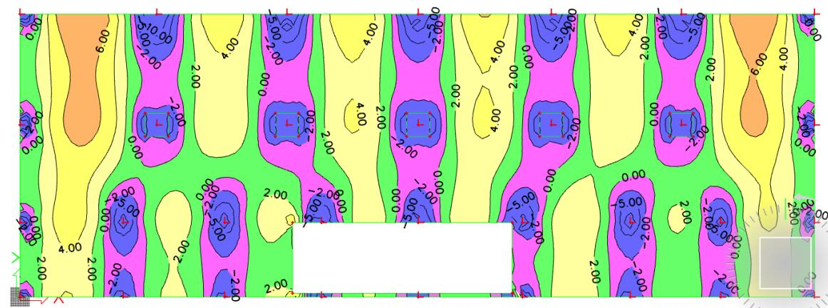
Slika 6.7 Potrebna površina armature  $A_s$  ( $\text{cm}^2/\text{m}$ ) u x smjeru
