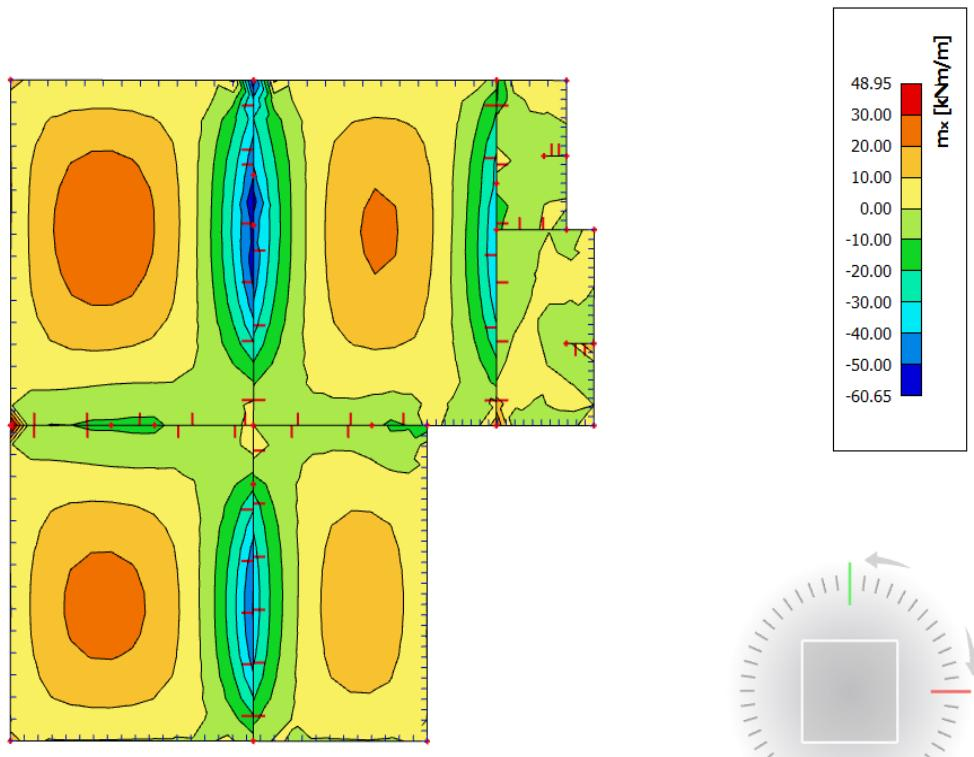
*Slika 6.3. Prikaz momenata savijanja u polju  $M_x$  – GSN2*
