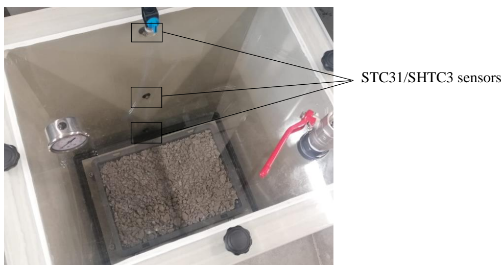
Fig. 32. Sensors inside chamber
