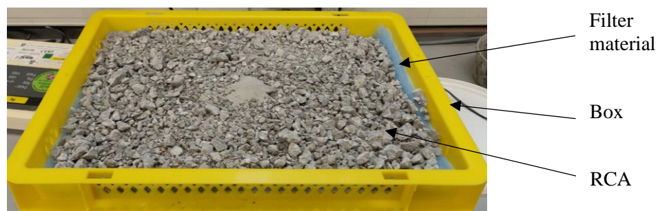
Fig. 27. RCA prepared for CO 2 curing.
