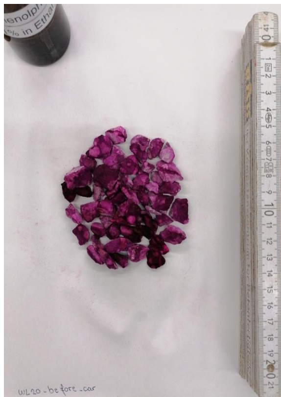
Fig. 19. Phenolphthalein test results before CO 2 curing for experiment WL20.
