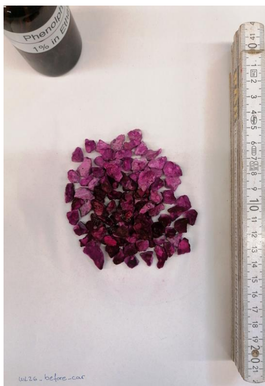
Fig. 37. Phenolphthalein test results before CO 2 curing for experiment WL26.
