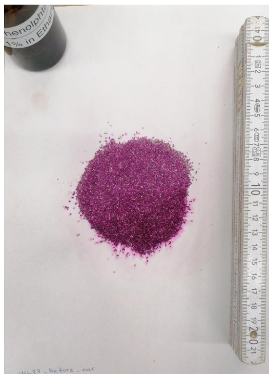
Fig. 40. Phenolphthalein test results before CO 2 curing for experiment WL27.
