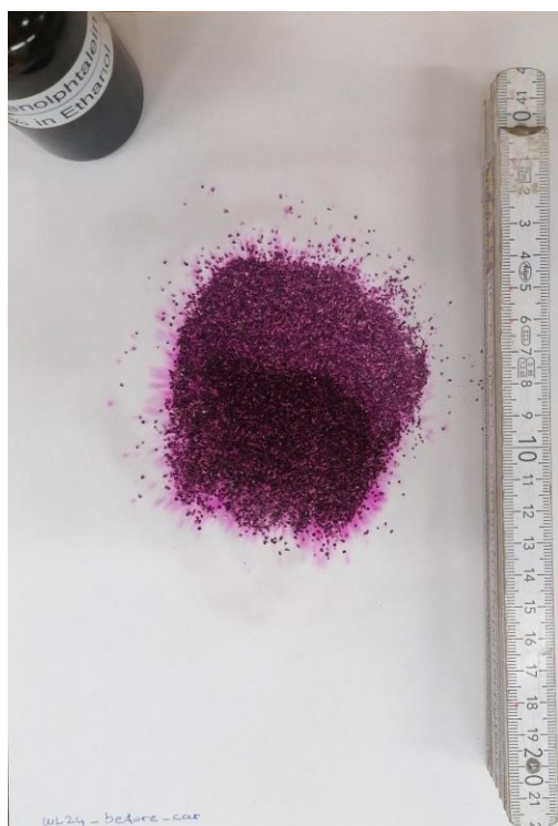
Fig. 31. Phenolphthalein test results before CO 2 curing for experiment WL24.
