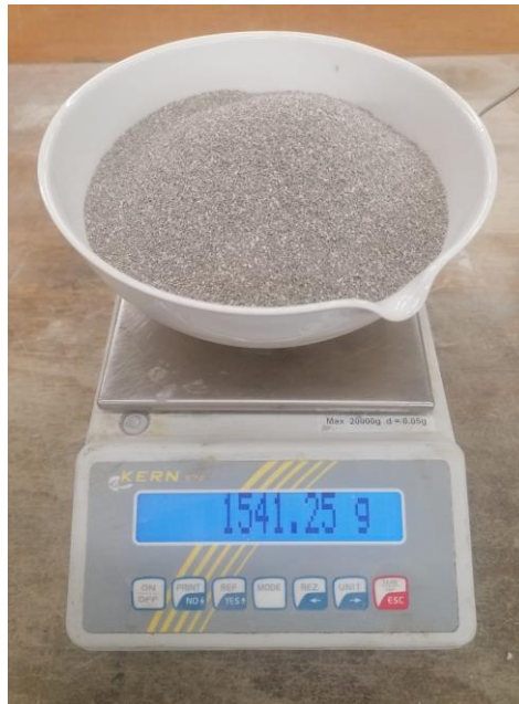
Fig. 33. Mass measurement during moisture content testing
