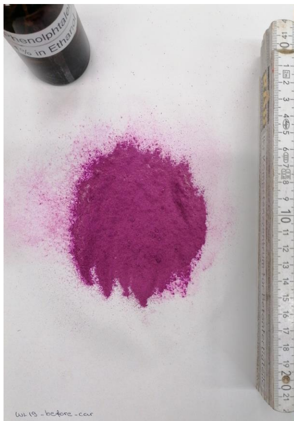
Fig. 16. Phenolphthalein test results before CO 2 curing for experiment WL19.
