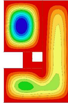
Progibi ploča. U_z (mm) – GSU – 2 ( \delta_{\max,d} \leq L/1250 )
