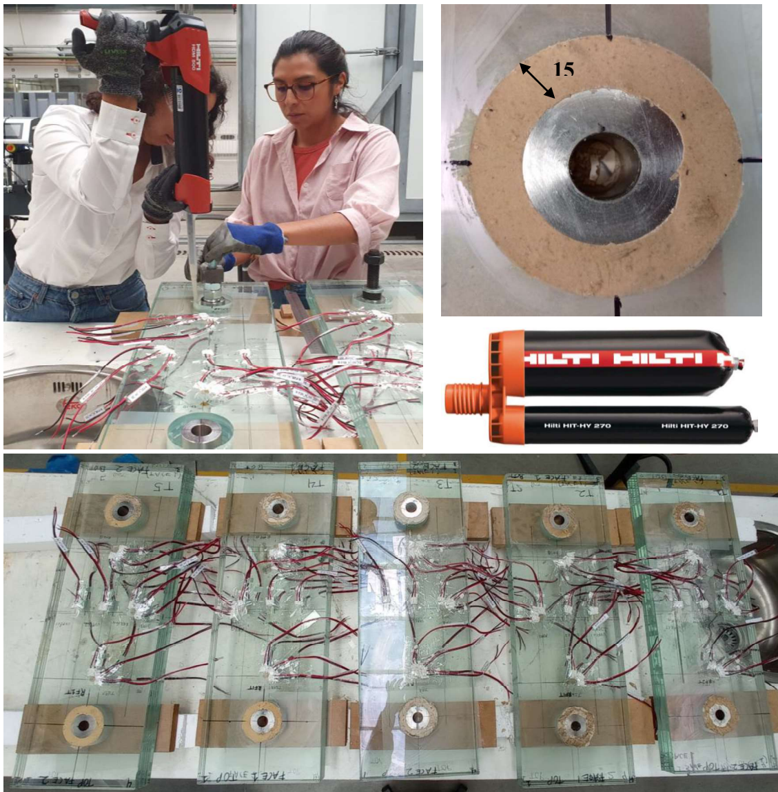
Figure 3.12 – Details regarding the grout application [7]
