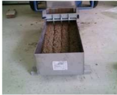
Fig. 6 L-box: SCLC 4 - sticky mixture
