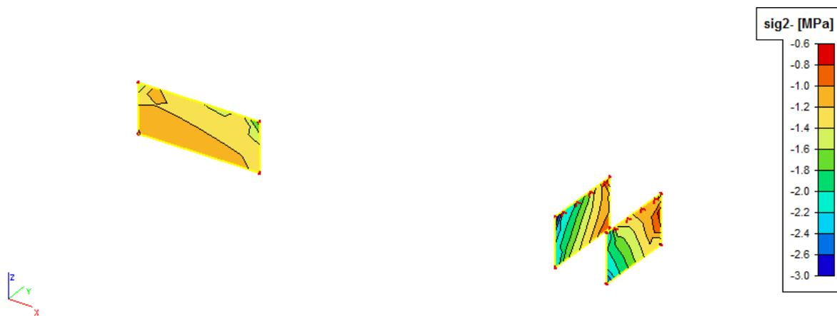
**Crtež 8.19.** Naprezanja u zidu  $\sigma_c$ , GSU-2:  $1,0 \cdot (G_0 + G) + 0,3Q$
