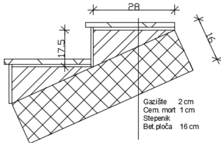
$$\operatorname{tga} = v_{st} / \dot{s}_{st} = 17,5 / 28 = 0,625 ; \alpha = 32,0^\circ$$
