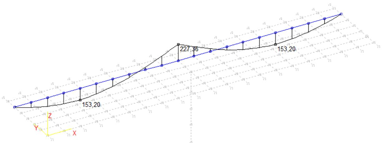
Slika 9.:Dodatno stalno-Poprečne sile  $T_z$  (Kn)
