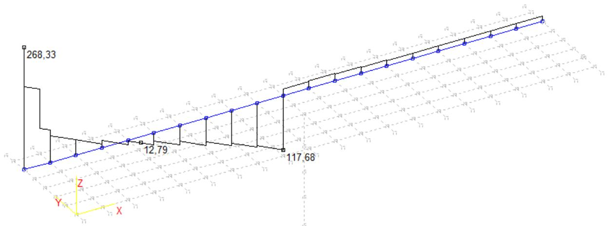
**MJERODAVNE SILE ZA DIMENZIONIRANJE JEDNOG UZDUŽNOG NOSAČA**
