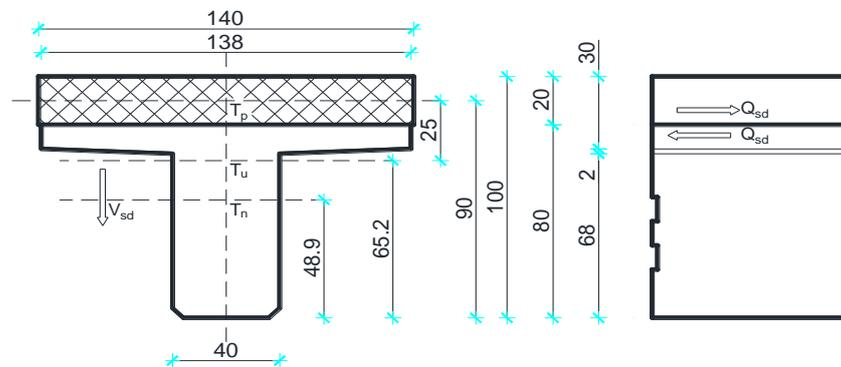
$$\left. \begin{aligned} A_n &= 0.426 \text{ m}^2 & h_{t,n} &= 0.489 \text{ m} \\ A_{pl} &= 0.280 \text{ m}^2 & h_{t,pl} &= 0.90 \text{ m} \end{aligned} \right\} A_u = 0.706 \text{ m}^2 \quad h_{t,u} = 0.652 \text{ m}$$
