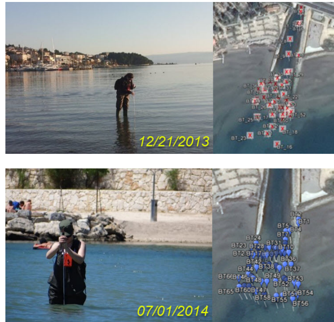
FIGURE 4.5: Velocity measurements procedure and the recorded positions for the winter (up) and summer (down) measuring campaigns.
