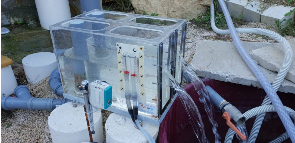
FIGURE A.18: V-Notch weirs for discharge measurement.
