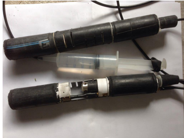
FIGURE A.21: Borehole packers.
