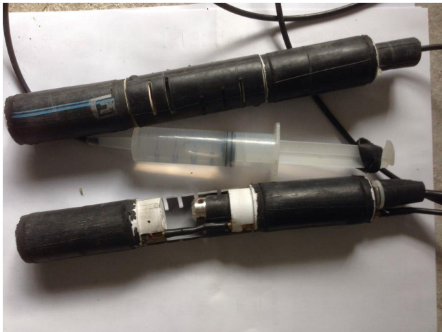
FIGURE A.21: Borehole packers.
