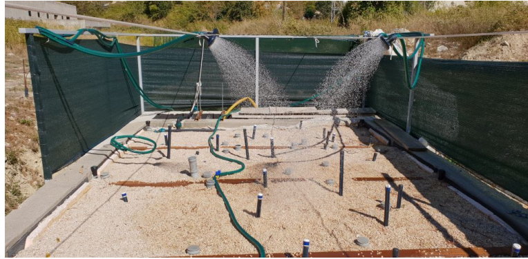
FIGURE A.15: Photography of rain simulation by two shower heads.
