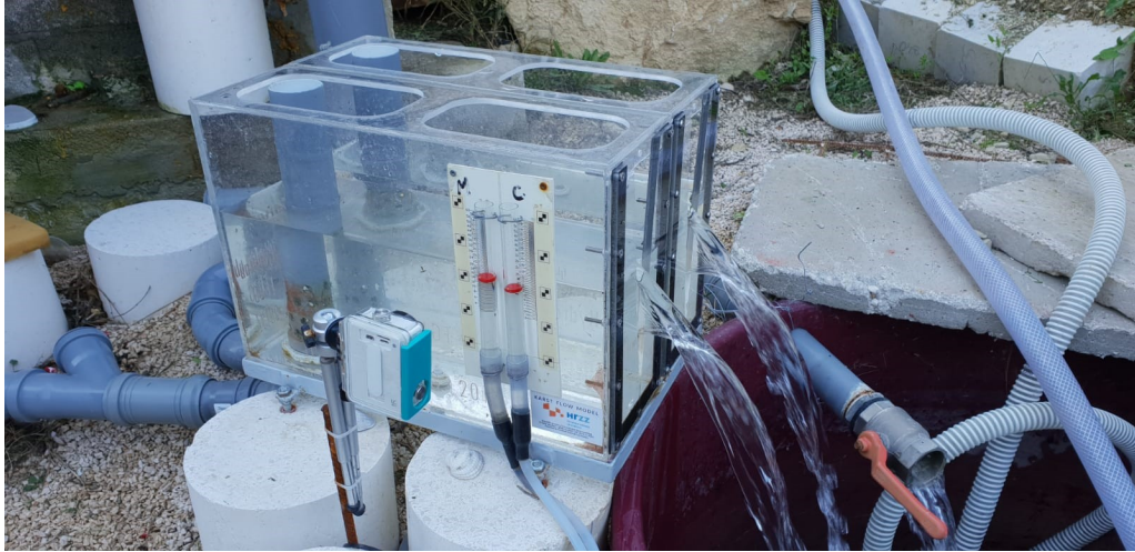
FIGURE A.18: V-Notch weirs for discharge measurement.
