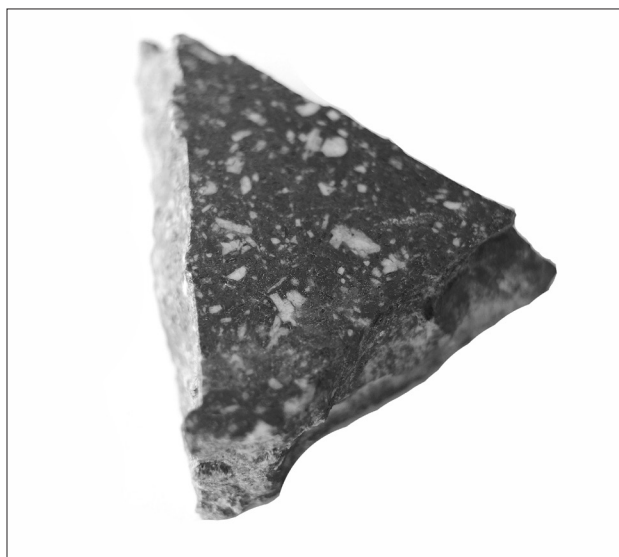
Fig. 3. Porfido Rosso Antico: upside-down view of a thin slab (thickness 10 mm) with oblique edges
