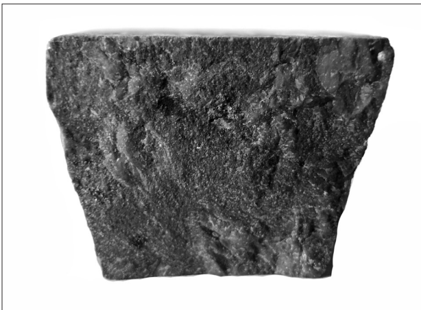
Fig. 4. Porfido Serpentino Verde: listel with trapezoidal section (thickness 14 mm)
