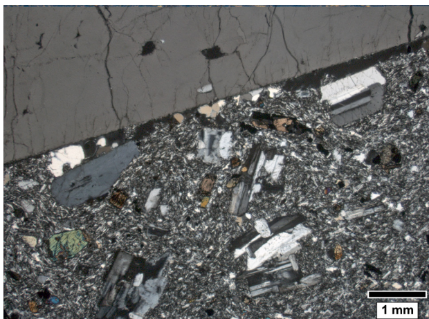
Fig. 10. Photomicrograph of trachyte from Drachenfels (Nr. 2049). Sanidine inclusion in the fine-grained matrix of plagioclase, quartz, pyroxene, biotite and opaque minerals under crossed polarized light (photo: V. Ruppiniè)
