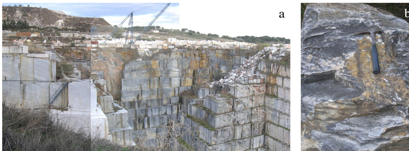
Fig. 1a. One of the active quarries in the south of the EA district. b. Detail of the foliation developed on a grey marble outcrop
