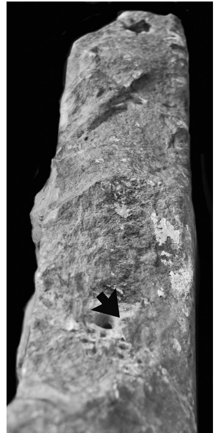
Fig. 10. Top right side of the Tiberius Relief with pre-existing drill hole: arrow by J. Podany, indicating area from which marble samples were taken (photo: J. Pollini)
