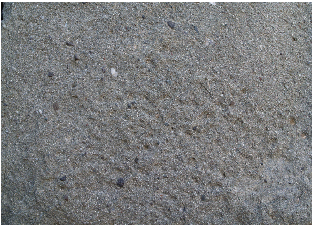
Fig. 7. Volcaniclastic sandstone, macroscopic appearance (photo: B. Djurić)
