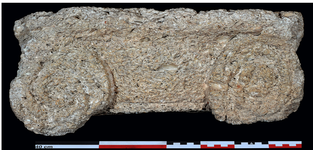
Fig. 11. Small Ionic capital of pure lumachella limestone from one of the fortification's entrance zones (photo: B. Djurić)
