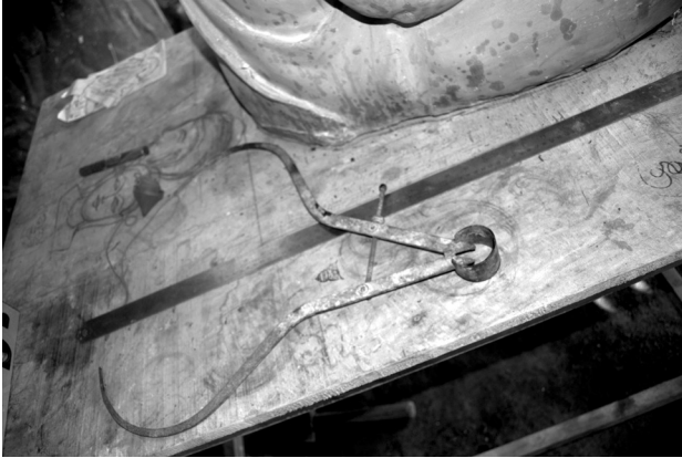
Fig. 23. Caliper and triangulation process in a workshop of Mahabalipuram, India (photo: S. Moureaud)
