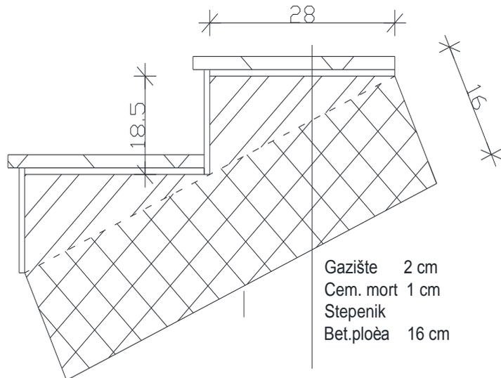
$$\operatorname{tg}\alpha = v_{st}/\check{s}_{st} = 18,5/28 = 0,6607 ; \alpha = 33,45^{\circ}$$
