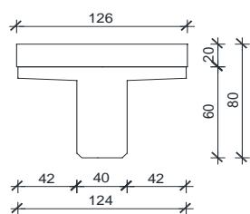
$$\begin{aligned}A &= 0.59 \text{ m}^2 \\I_y &= 0.0278 \text{ m}^4 \\I_z &= 0.0503 \text{ m}^4 \\E &= 34000 \text{ MPa}\end{aligned}$$
