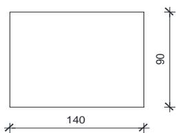
$$\begin{aligned}A &= 1.26 \text{ m}^2 \\I_y &= 0.085 \text{ m}^4 \\I_z &= 0.0205 \text{ m}^4 \\E &= 34000 \text{ MPa}\end{aligned}$$
