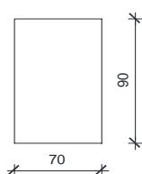
$$\begin{aligned}A &= 0.63 \text{ m}^2 \\I_y &= 0.0425 \text{ m}^4 \\I_z &= 0.0257 \text{ m}^4 \\E &= 34000 \text{ MPa}\end{aligned}$$
