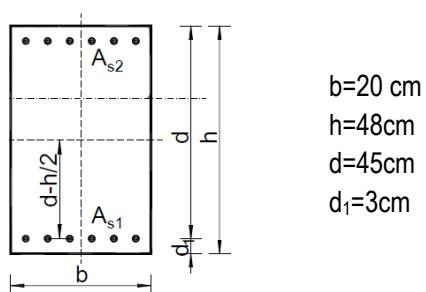
$$\begin{aligned} b &= 20 \text{ cm} \\ h &= 48 \text{ cm} \\ d &= 45 \text{ cm} \\ d_1 &= 3 \text{ cm} \end{aligned}$$
