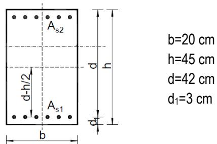
$$\begin{aligned} b &= 20 \text{ cm} \\ h &= 45 \text{ cm} \\ d &= 42 \text{ cm} \\ d_1 &= 3 \text{ cm} \end{aligned}$$
