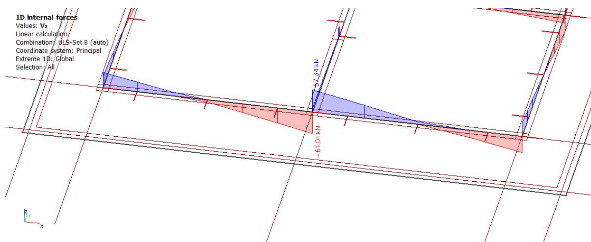
Slika 63 Dijagram poprečnih sila  $V_z$  na gredama**Poprečni presjek grede:**
