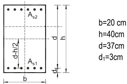
$$\begin{aligned} b &= 20 \text{ cm} \\ h &= 40 \text{ cm} \\ d &= 37 \text{ cm} \\ d_1 &= 3 \text{ cm} \end{aligned}$$
