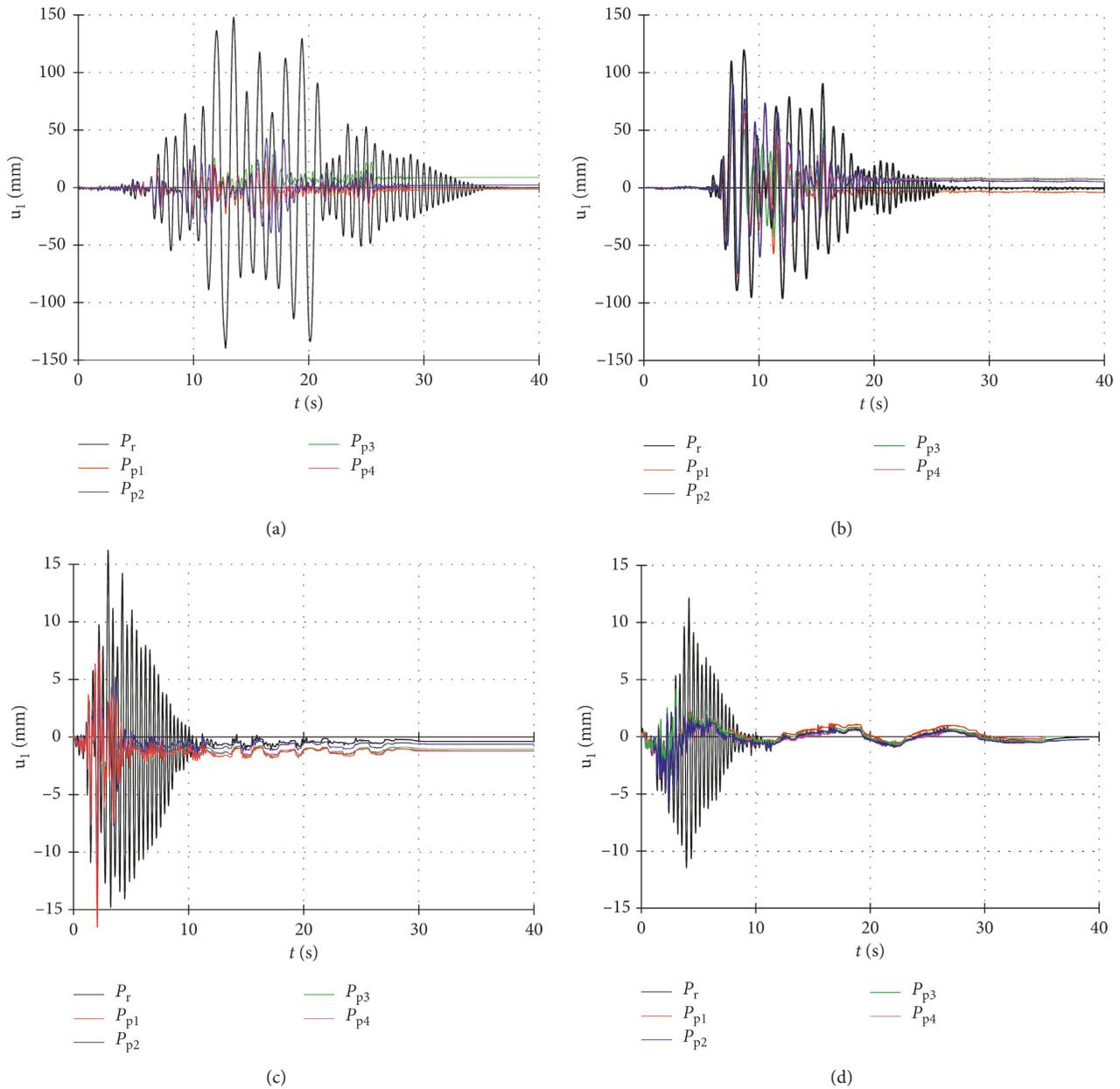
FIGURE 11: Horizontal displacement of the mass center at the column top ( $u_1$ ). (a) Artificial accelerogram (AA). (b) Accelerogram Petrovac (AP). (c) Accelerogram Ston (AS). (d) Accelerogram B. Luka (ABL).
