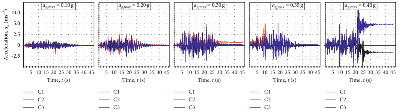
FIGURE 11: Horizontal acceleration of the column top.
