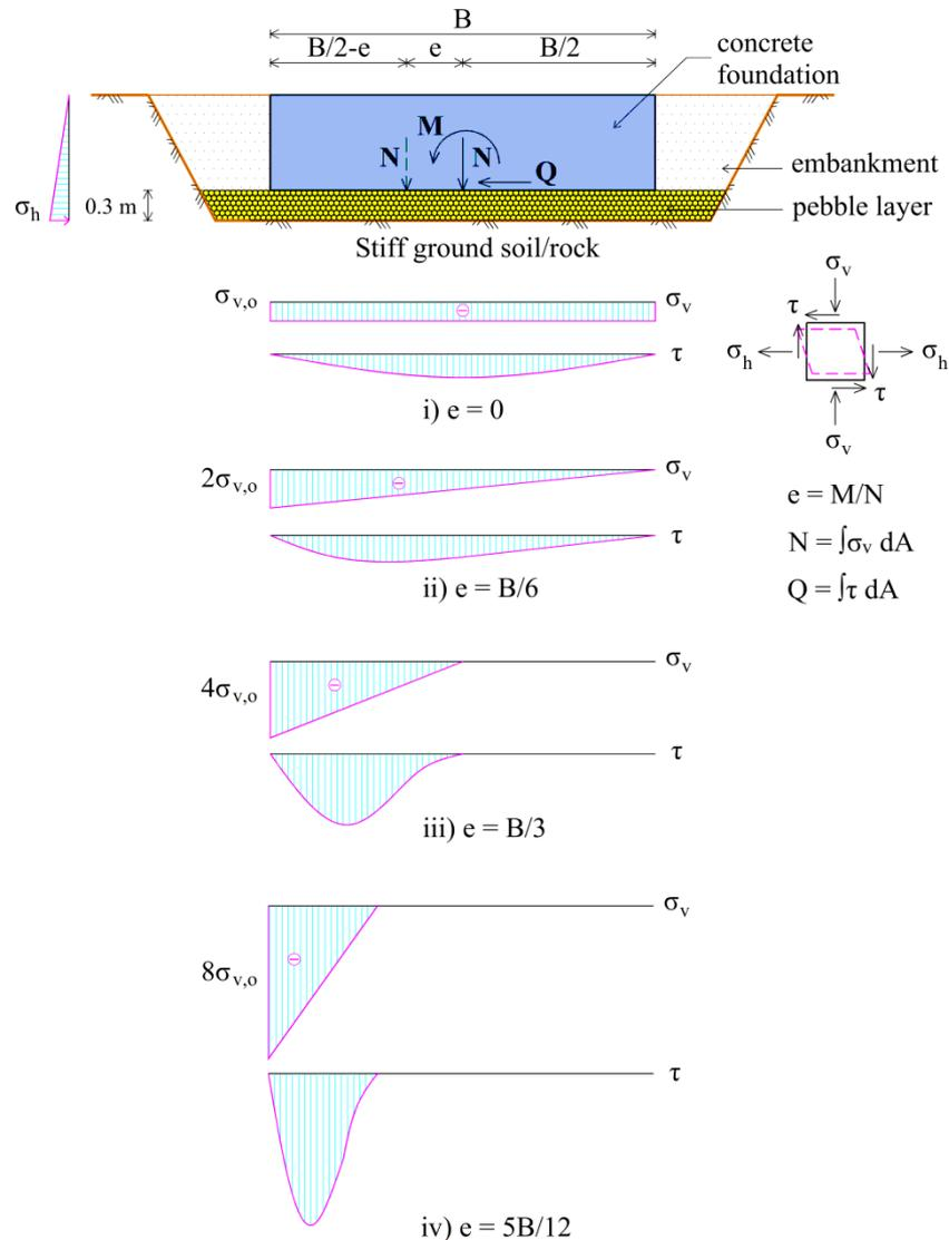
Figure 1 – Scheme of vertical normal stress and shear-stress distribution below the foundation
