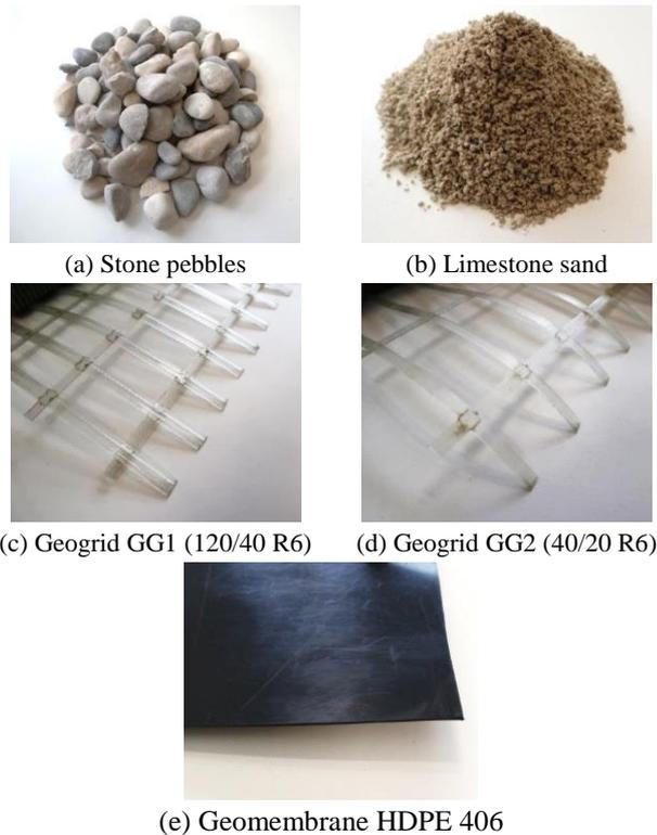
Fig. 2 Adopted materials/elements for the aseismic layer
