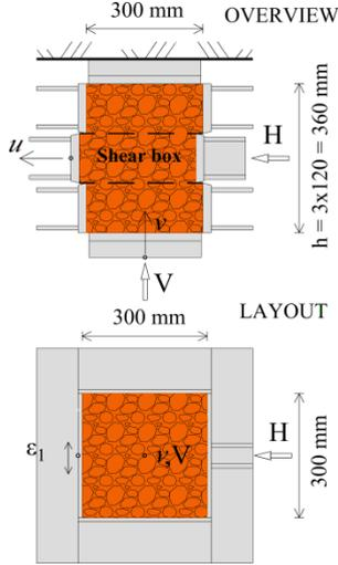
Figure 6 – Measured quantities during direct shear testing
