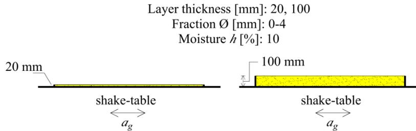
Figure 2.1 Considered limestone sand aseismic layers
