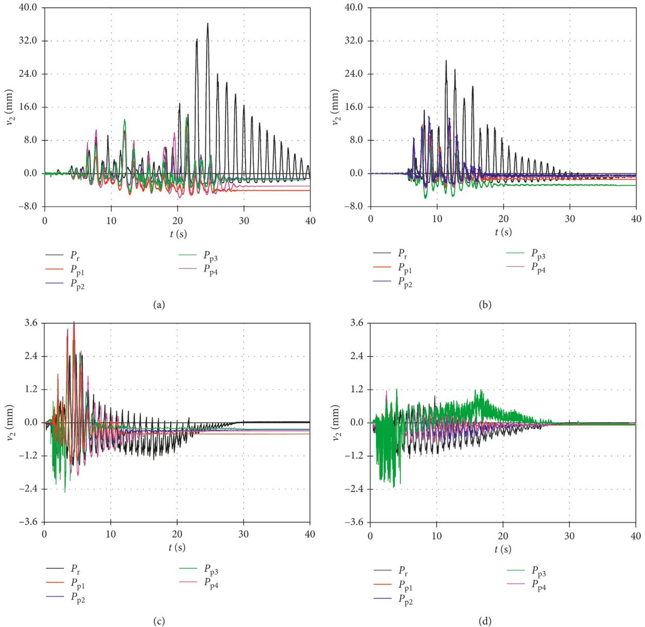
FIGURE 19: Foundation vertical displacement at the left edge ( $v_2$ ) for MSSB. (a) Artificial accelerogram (AA). (b) Accelerogram Petrovac (AP). (c) Accelerogram Ston (AS). (d) Accelerogram B. Luka (ABL).
