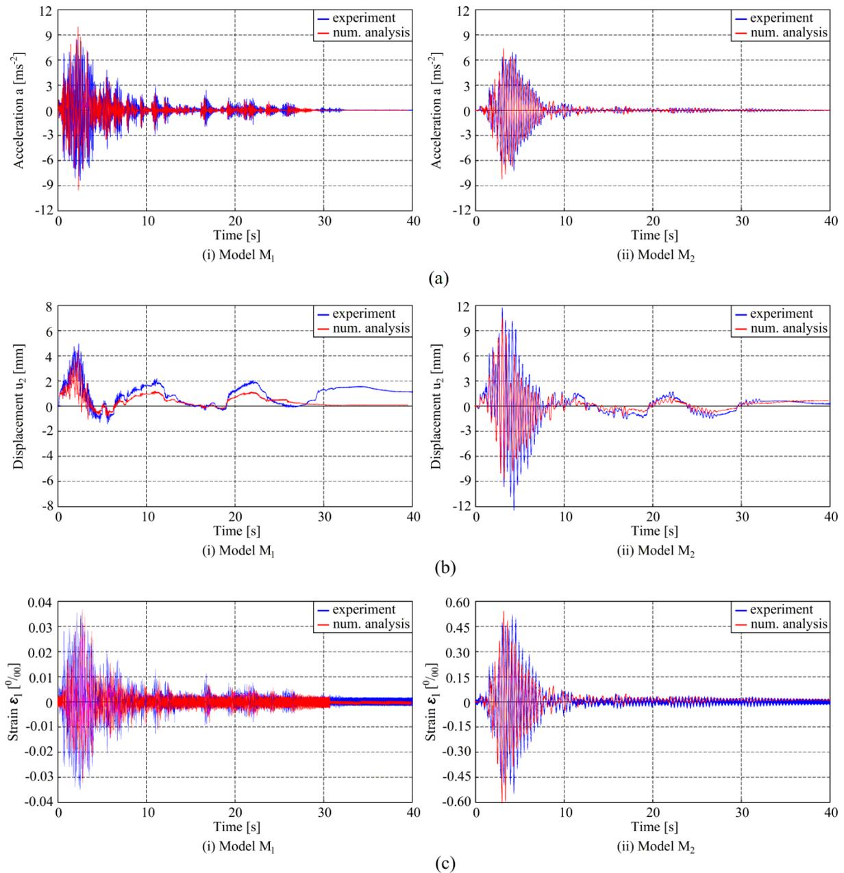
Figure 18 – Comparison of experimentally determined and numerically obtained results for applied ABL accelerogram ( $PGA = 0.3\text{ g}$ ): (a) Horizontal acceleration  $a$  of the mass at the column top, (b) Horizontal displacement  $u_2$  of the mass at the column top, (c) Vertical strain  $\varepsilon_1$  on the right bottom side of the steel column
