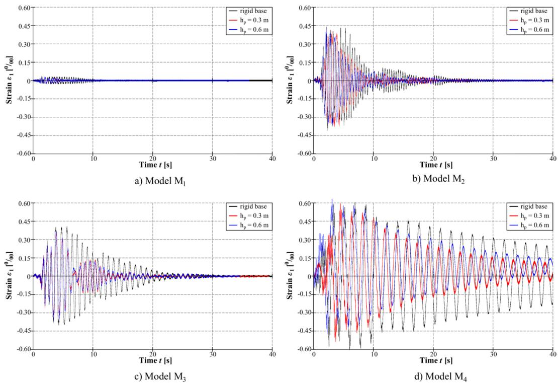
Figure 13 - Vertical strain on the right bottom side of the steel column  $\epsilon_1$  for accelerogram AS
