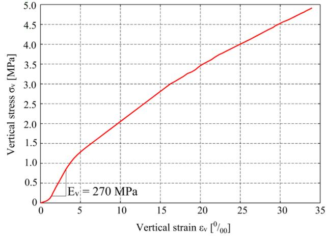
Figure 7 – Normal stress–normal strain curve due to testing of a stone pebble in shear box subjected to normal stress only (without shear force)
