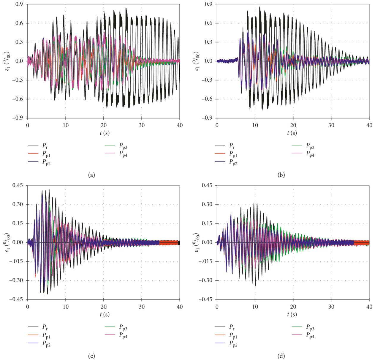
FIGURE 17: Vertical strain on the right bottom side of the steel column ( $\varepsilon_1$ ) for MSSB. (a) Artificial accelerogram (AA). (b) Accelerogram Petrovac (AP). (c) Accelerogram Ston (AS). (d) Accelerogram B. Luka (ABL).
