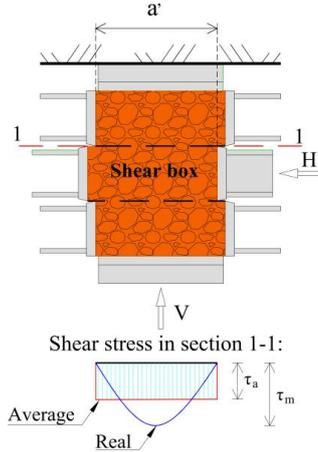
Figure 10 – Shear stress distribution in section 1-1
