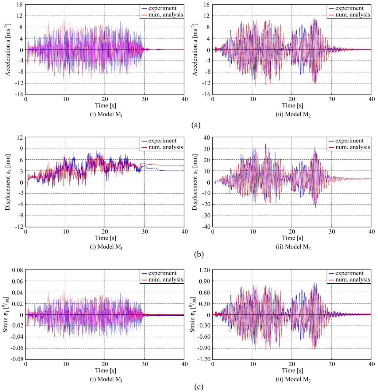
Figure 3.8. Comparison of experimentally determined and numerically obtained results for applied AA accelerogram ( $PGA = 0.3\text{ g}$ ): (a) Horizontal acceleration  $a$  of the mass at the column top; (b) Horizontal displacement  $u_2$  of the mass at the column top; (c) Vertical strain  $\varepsilon_1$  on the right bottom side of the steel column
