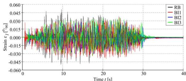
Fig. 15 Vertical strain on the right bottom side of the steel column  $\varepsilon_l$  of model  $M_1$  for accelerogram AA
