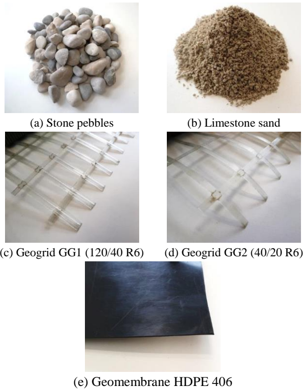
Fig. 2 Adopted materials/elements for the aseismic layer
