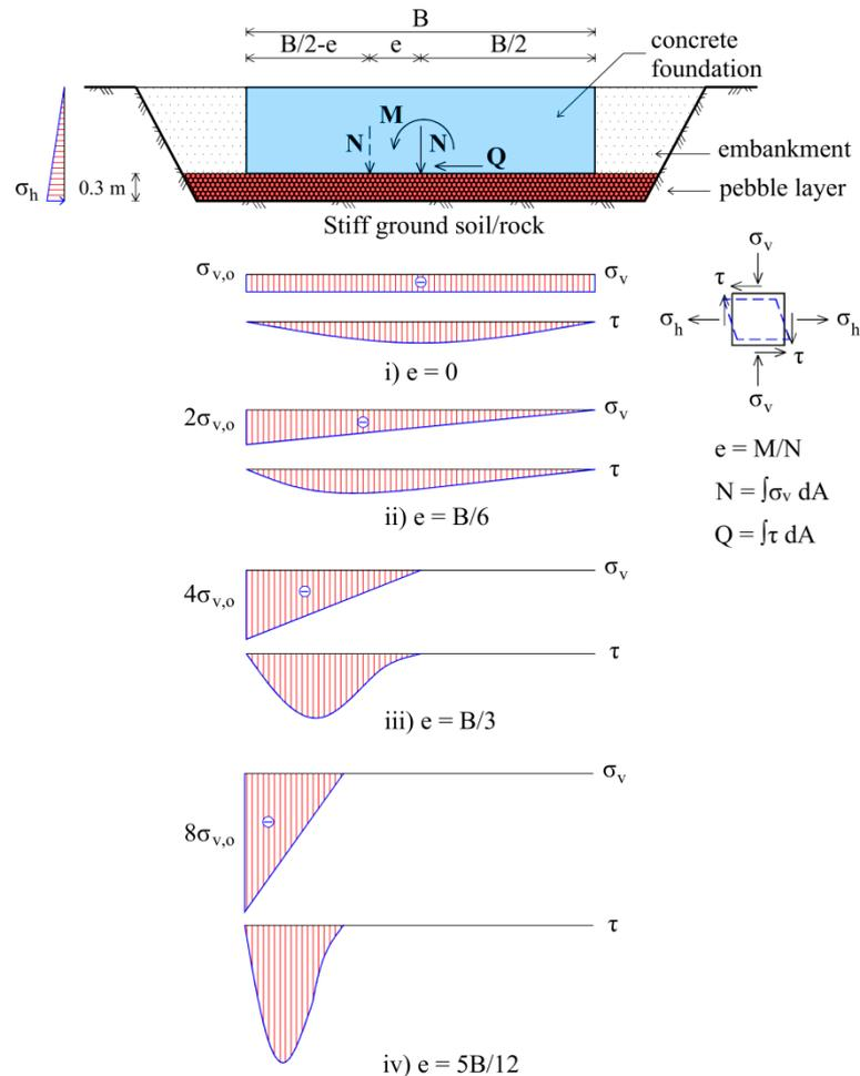
Figure 3.1. The distribution scheme of normal and shear stress below the foundation
