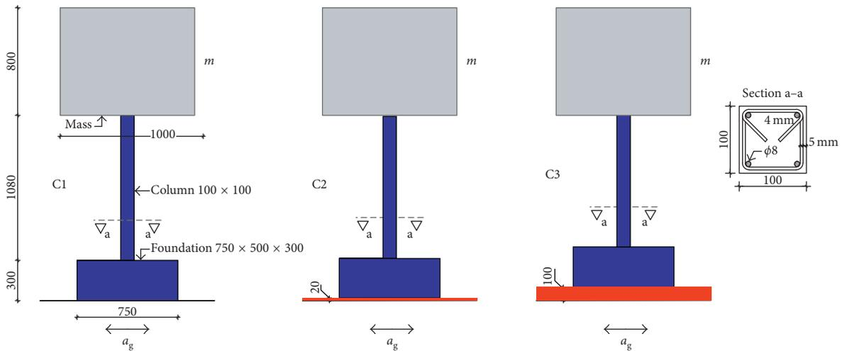
FIGURE 2: Basic data of the tested column.
