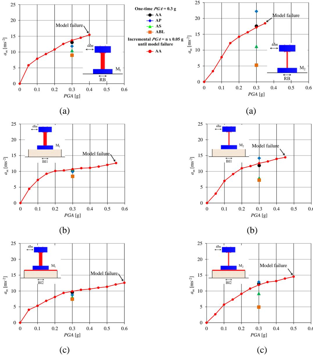
Figure 2.18 The peak acceleration  $a_m$  of the  $M_1$ : (a)  $M_1$  on RB; (b)  $M_1$  on B11; (c)  $M_1$  on B12
