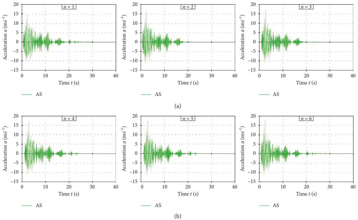
FIGURE 30: Horizontal acceleration  $a$  for repeated excitation AS.
