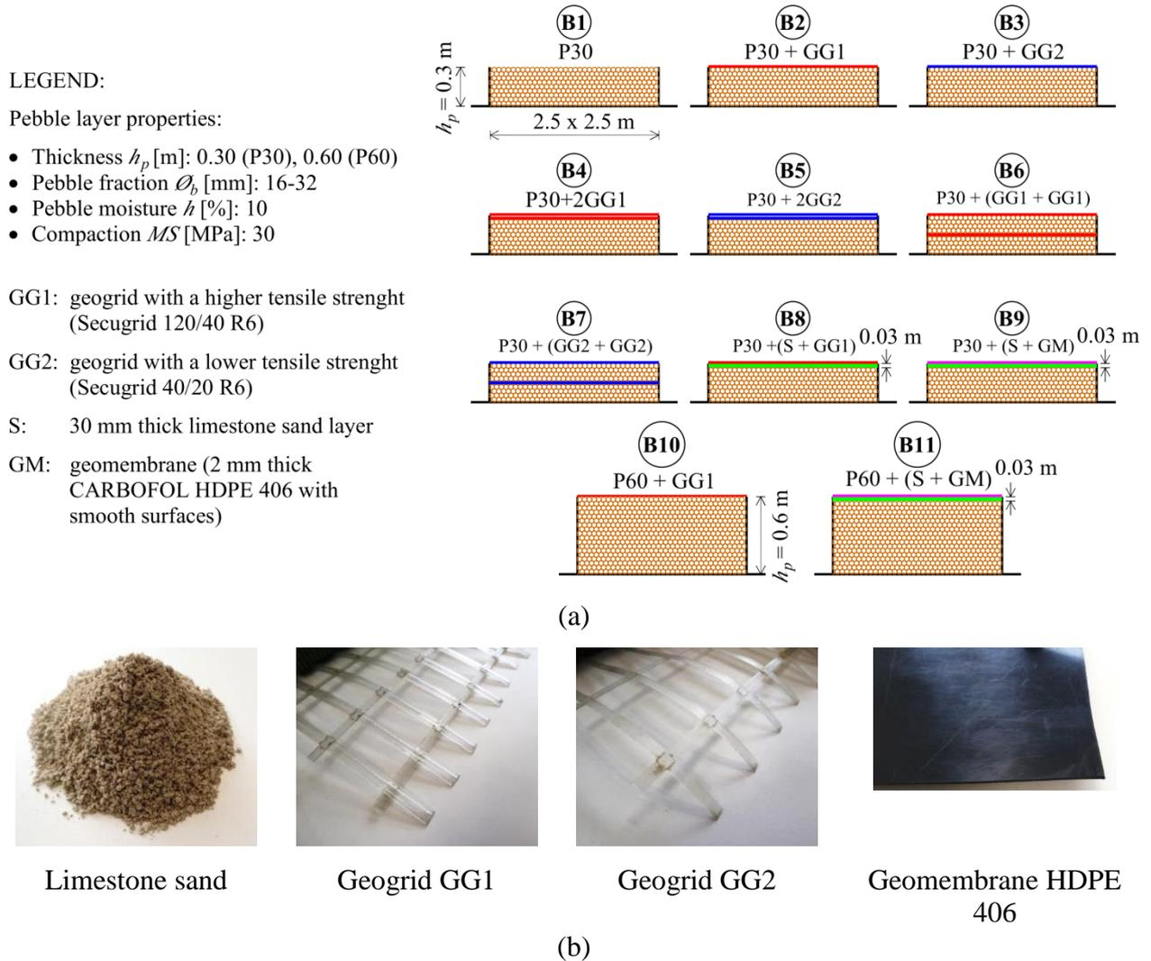
Figure 2.3 ASL-3 aseismic layers: (a) Composite seismic base isolations considered in this study; (b) Adopted materials for the sliding layer
