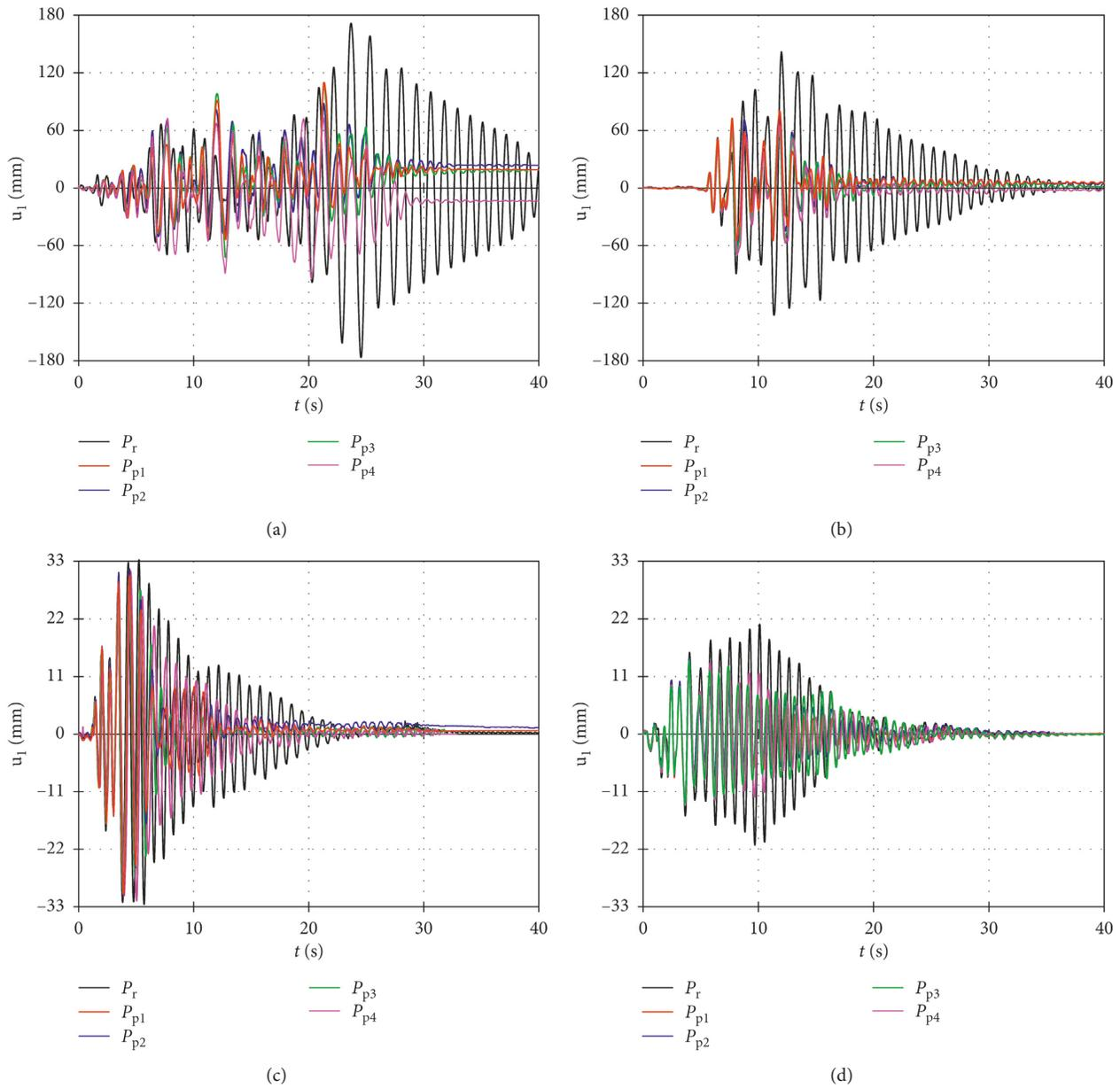
FIGURE 16: Horizontal displacement of the mass center at the column top ( $u_1$ ) for MSSB. (a) Artificial accelerogram (AA). (b) Accelerogram Petrovac (AP). (c) Accelerogram Ston (AS). (d) Accelerogram B. Luka (ABL).
