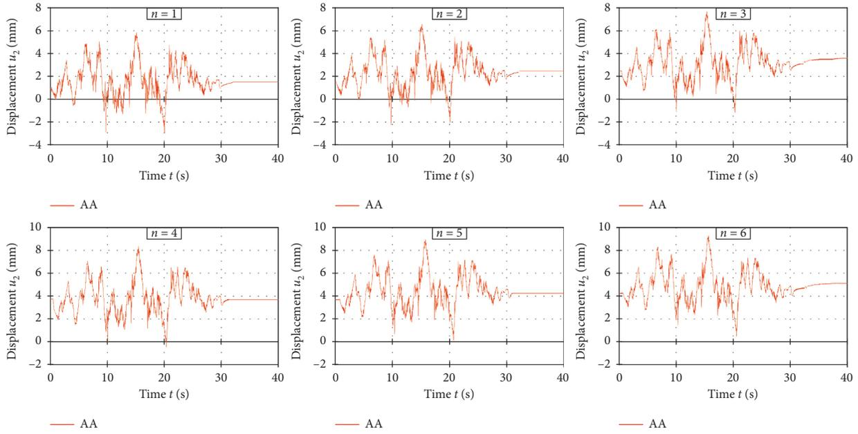
FIGURE 29: Horizontal displacement  $u_2$  for repeated excitation AA.
