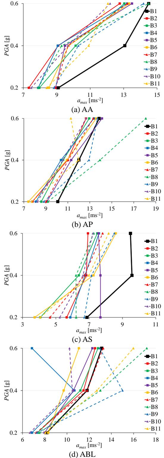
Fig. 6 Peak horizontal acceleration of the mass center  $a_{max}$
