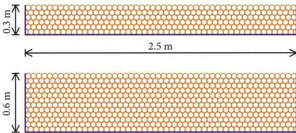
FIGURE 2: Used thicknesses of pebble layer.
