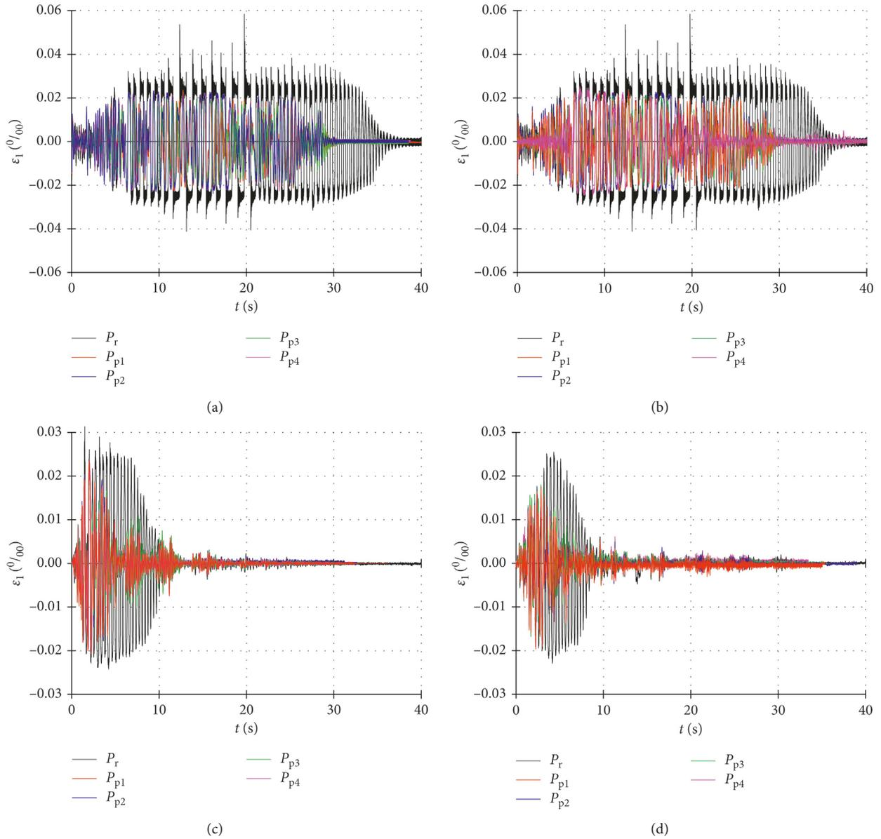
FIGURE 12: Vertical strain on the right bottom side of the steel column ( $\varepsilon_1$ ) for MSB. (a) Artificial accelerogram (AA). (b) Accelerogram Petrovac (AP). (c) Accelerogram Ston (AS). (d) Accelerogram B. Luka (ABL).
