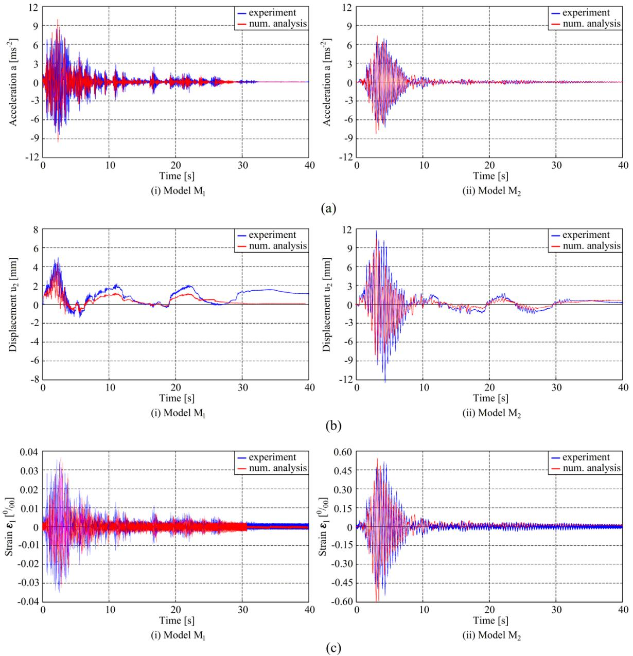
Figure 3.9. Comparison of experimentally determined and numerically obtained results for applied ABL accelerogram ( $PGA = 0.3 \text{ g}$ ): (a) Horizontal acceleration  $a$  of the mass at the column top; (b) Horizontal displacement  $u_2$  of the mass at the column top; (c) Vertical strain  $\varepsilon_1$  on the right bottom side of the steel column
