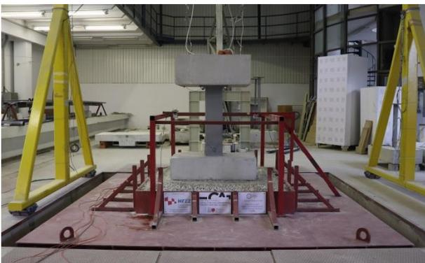
(a) Experimental setup on shake table with model  $M_1$  based on BI2 isolation
