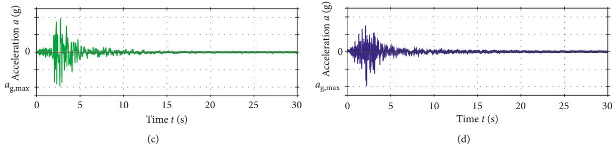
FIGURE 6: Applied horizontal base accelerations ( $a_{g,max}$  scaled to 0.2 g for MSSB and 0.3 g for MSB). (a) Artificial accelerogram (AA). (b) N-S accelerogram of Petrovac earthquake (AP). (c) N-S accelerogram of Ston earthquake (AS). (d) N-S accelerogram of B. Luka earthquake (ABL).
