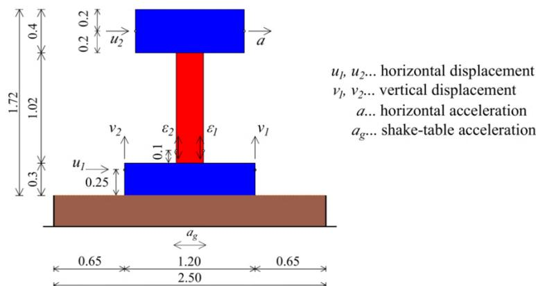
Figure 2.10 Measured quantities on the  $M_1, M_2, M_3,$  and  $M_4$  models on ASL-2 and ASL-3
