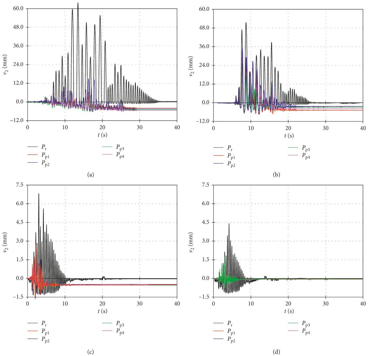
FIGURE 14: Vertical displacement at the left edge of the foundation ( $v_2$ ) for MSB. (a) Artificial accelerogram (AA). (b) Accelerogram Petrovac (AP). (c) Accelerogram Ston (AS). (d) Accelerogram B. Luka (ABL).
