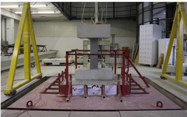
(a) Experimental setup on shake table with model M_1 based on BI2 isolation
