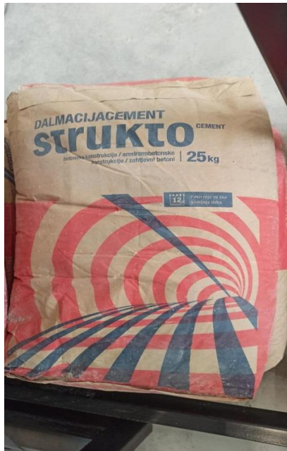
Slika 32 Cement CEM II/B-M (S-LL) 42,5N
