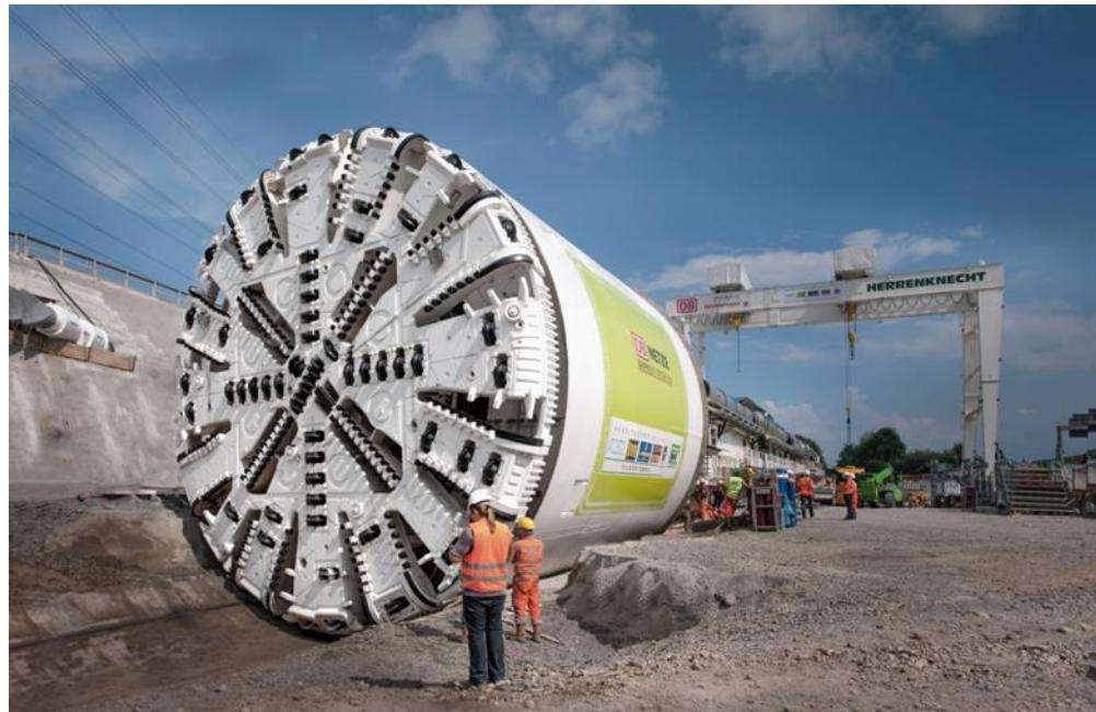
Slika 2.1: Herrenknecht Multi-Mode Tunnel Boring Machine [2]
