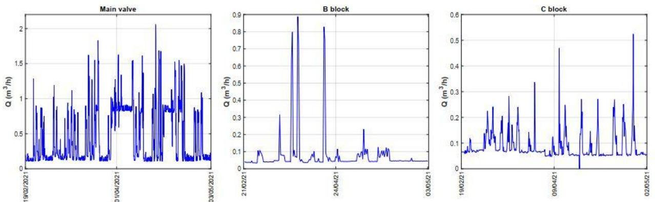
Slika 10.8. Mjerena potrošnja vode na tri uređaja (izvor: Deployment for Smart Building: Water Consumption Analysis)
