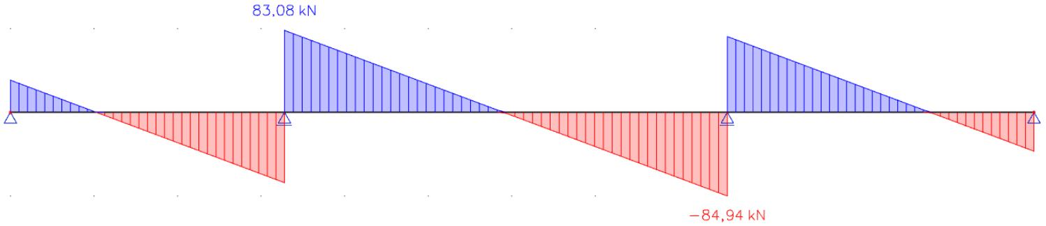
**C 30/37 ,  $V_{ed} = 84,94 \text{ kN}$**
