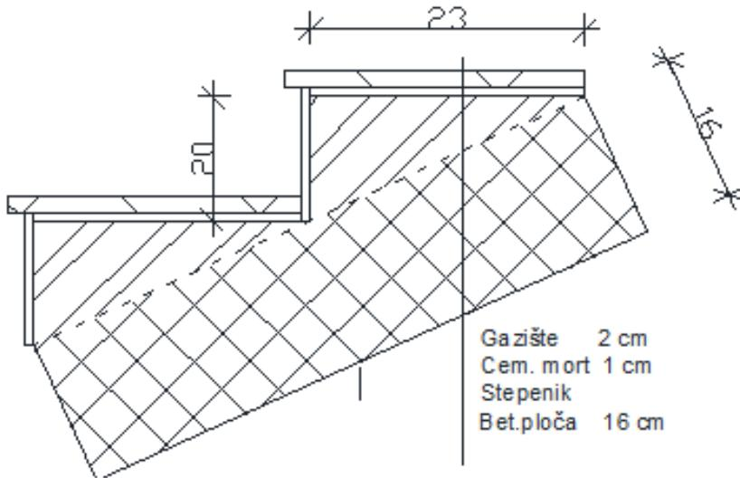
$$\operatorname{tg}\alpha = v_{st} / s_{st} = 20/25 = 0,8696 ; \alpha = 38,66^\circ$$
