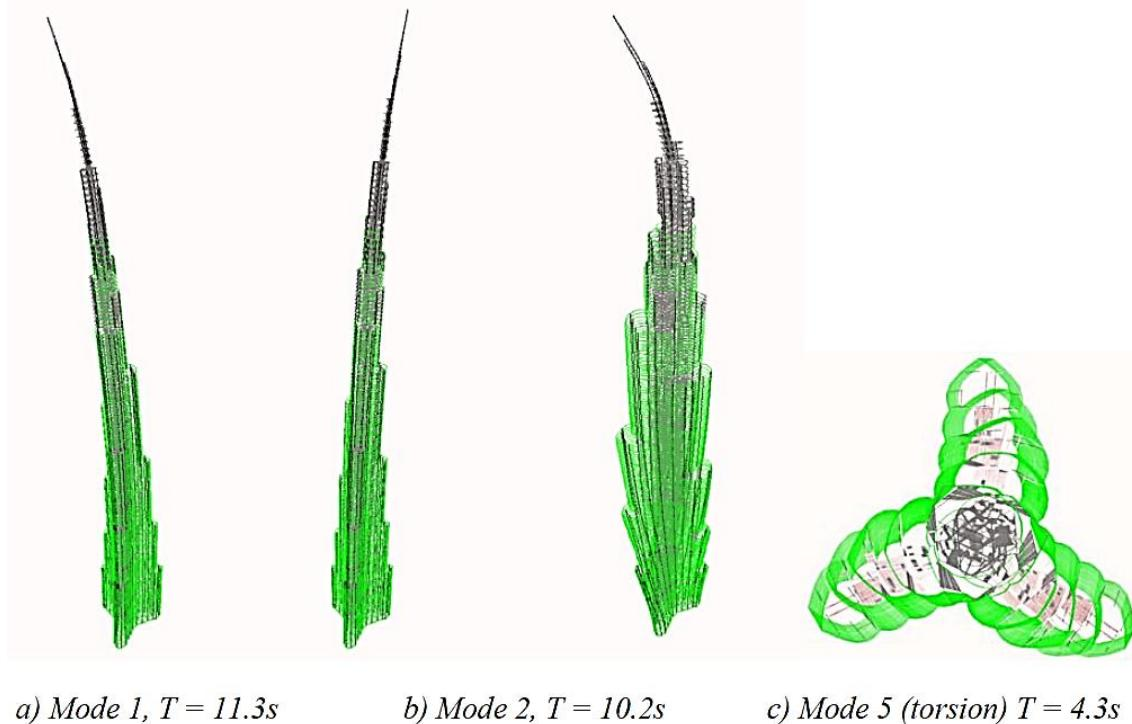
a) Mode 1,  $T = 11.3s$       b) Mode 2,  $T = 10.2s$       c) Mode 5 (torsion)  $T = 4.3s$
