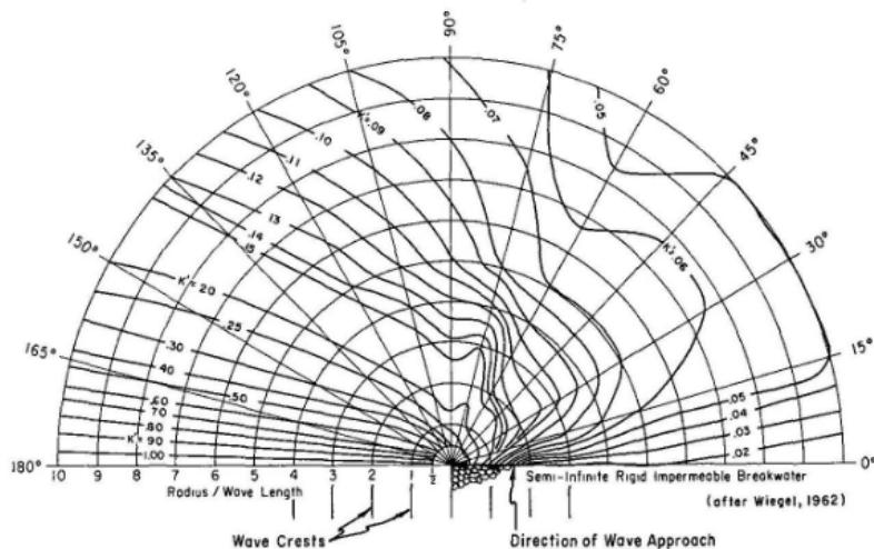
Figure 2-39. Wave Diffraction Diagram - 180° Wave Angle
