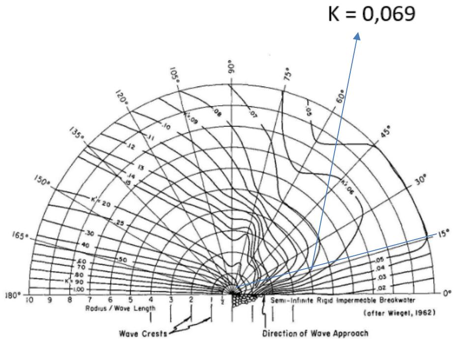
Figure 2-39. Wave Diffraction Diagram - 180° Wave Angle
