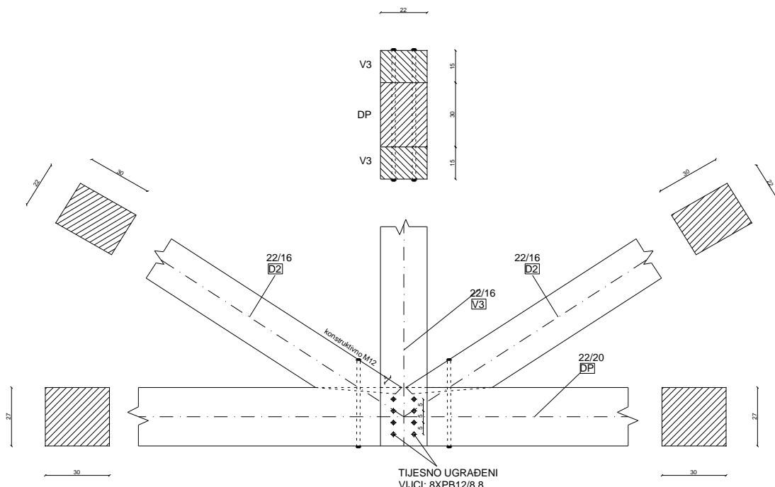
$$f_{c,a,d} = \frac{f_{c,0,d}}{\sqrt{\left(\frac{f_{c,0,d}}{2 \cdot f_{c,90,d}} \cdot \sin^2 \alpha\right)^2 + \left(\frac{f_{c,0,d}}{2 \cdot f_{v,d}} \cdot \sin \alpha \cdot \cos \alpha\right)^2 + \cos^4 \alpha}}$$
