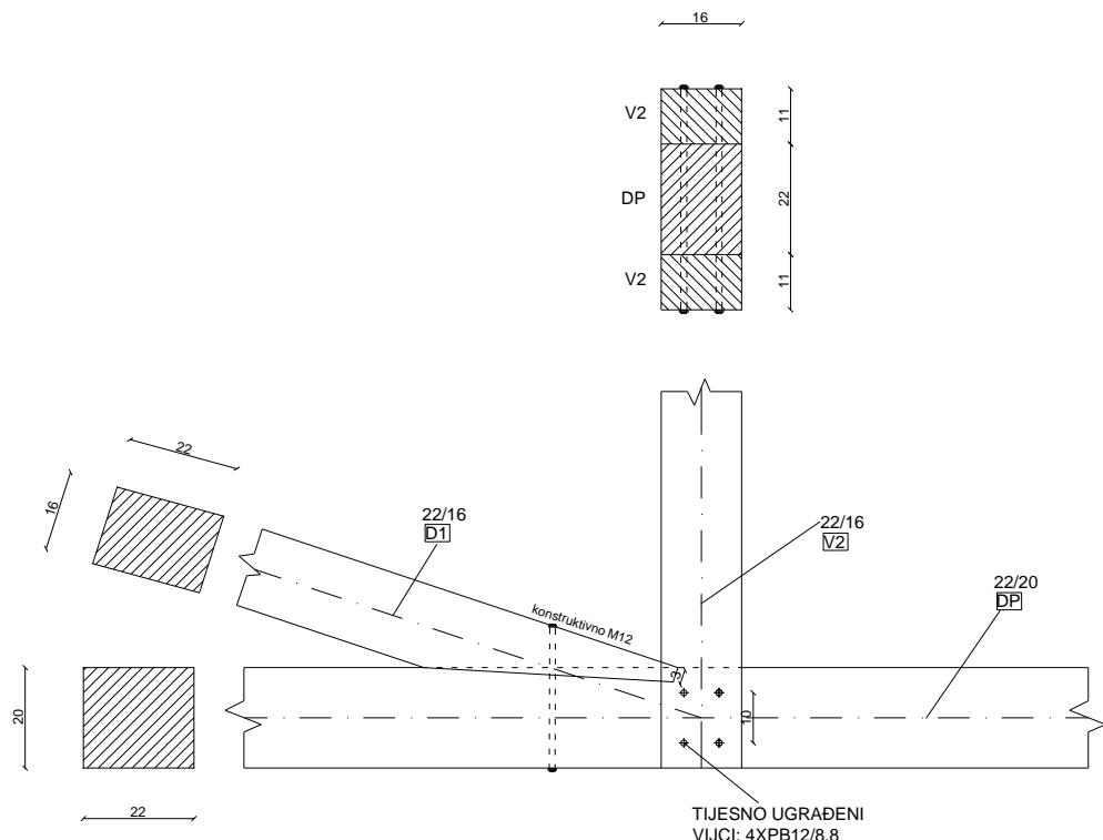
$$f_{c,a,d} = \frac{f_{c,0,d}}{\sqrt{\left(\frac{f_{c,0,d}}{2 \cdot f_{c,90,d}} \cdot \sin^2 \alpha\right)^2 + \left(\frac{f_{c,0,d}}{2 \cdot f_{v,d}} \cdot \sin \alpha \cdot \cos \alpha\right)^2 + \cos^4 \alpha}}$$
