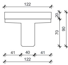
$$\begin{aligned}A &= 0.61 \text{ m}^2 \\I_y &= 0.039 \text{ m}^4 \\I_z &= 0.049 \text{ m}^4 \\E &= 34000 \text{ MPa}\end{aligned}$$
