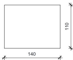
$$\begin{aligned}A &= 1.54 \text{ m}^2 \\I_y &= 0.1553 \text{ m}^4 \\I_z &= 0.2515 \text{ m}^4 \\E &= 34000 \text{ MPa}\end{aligned}$$
