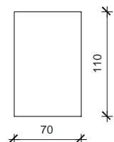
$$\begin{aligned}A &= 0.77 \text{ m}^2 \\I_y &= 0.0776 \text{ m}^4 \\I_z &= 0.0314 \text{ m}^4 \\E &= 34000 \text{ MPa}\end{aligned}$$
