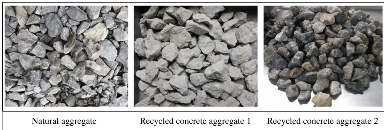
Fig. 1. Natural aggregate and different RC aggregates [9]
