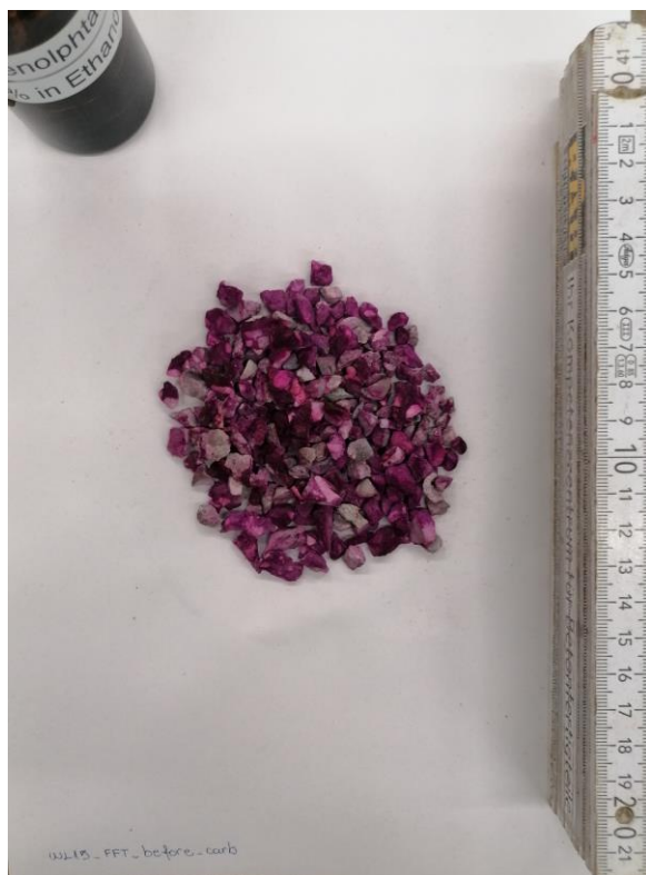
Fig. 4. Phenolphthalein test results before CO 2 curing for experiment WL15.
