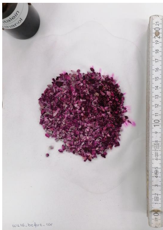
Fig. 7. Phenolphthalein test results before CO 2 curing for experiment WL16.
