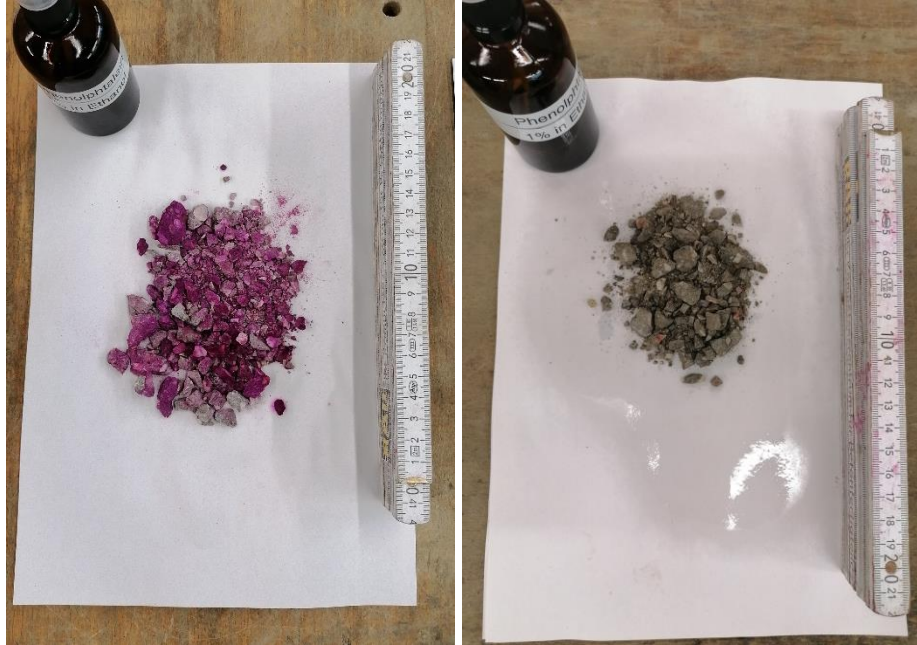
Fig. 9. Recycled concrete aggregate before carbonation (left) and after carbonation (right).
