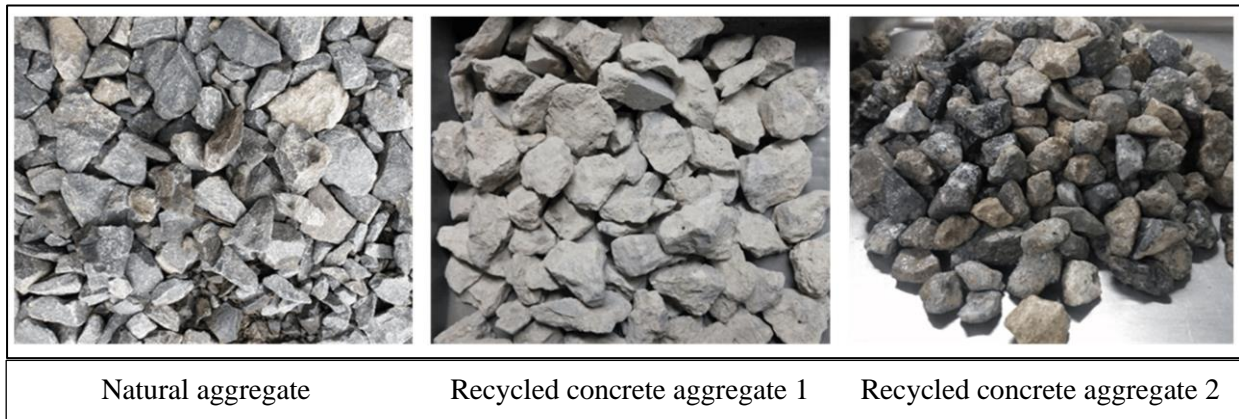
Fig. 1. Natural aggregate and different RC aggregates [9]
