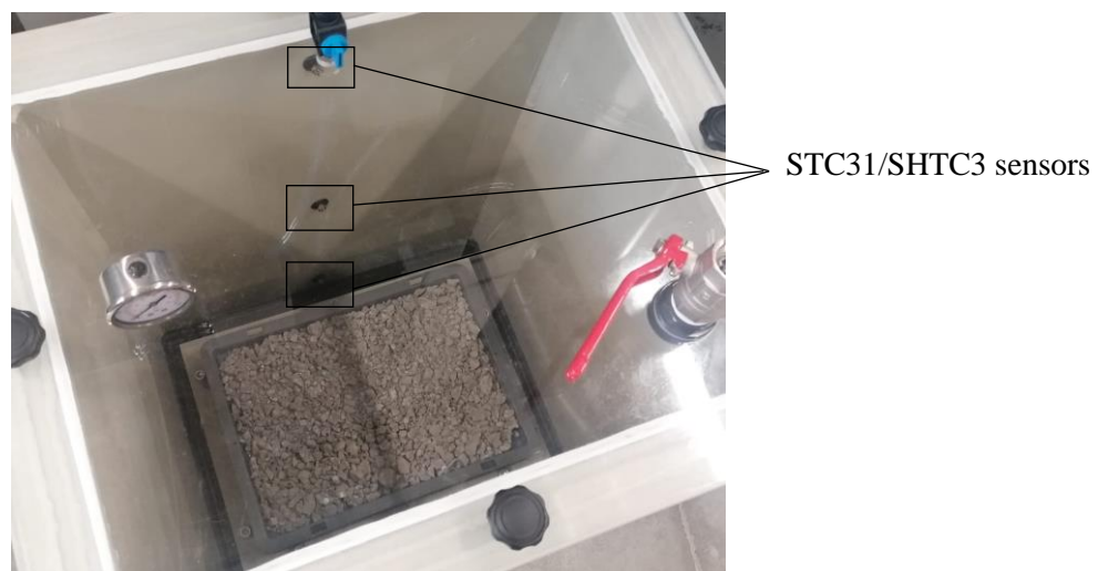
Fig. 32. Sensors inside chamber
