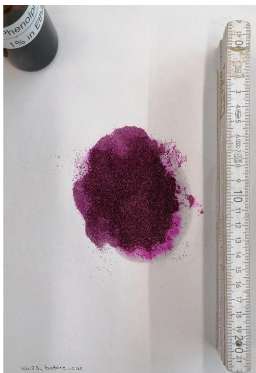
Fig. 28. Phenolphthalein test results before CO 2 curing for experiment WL23.
