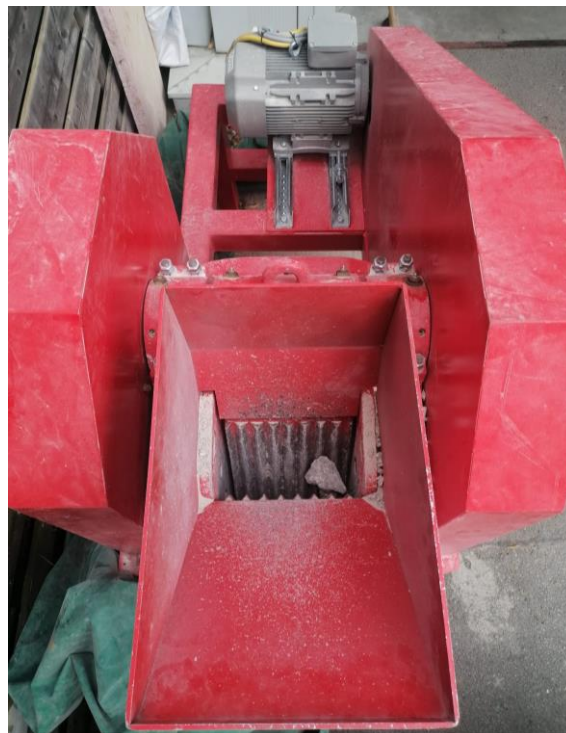
Fig. 22. Used jaw crusher with the swing jaw fixed at the upper position
