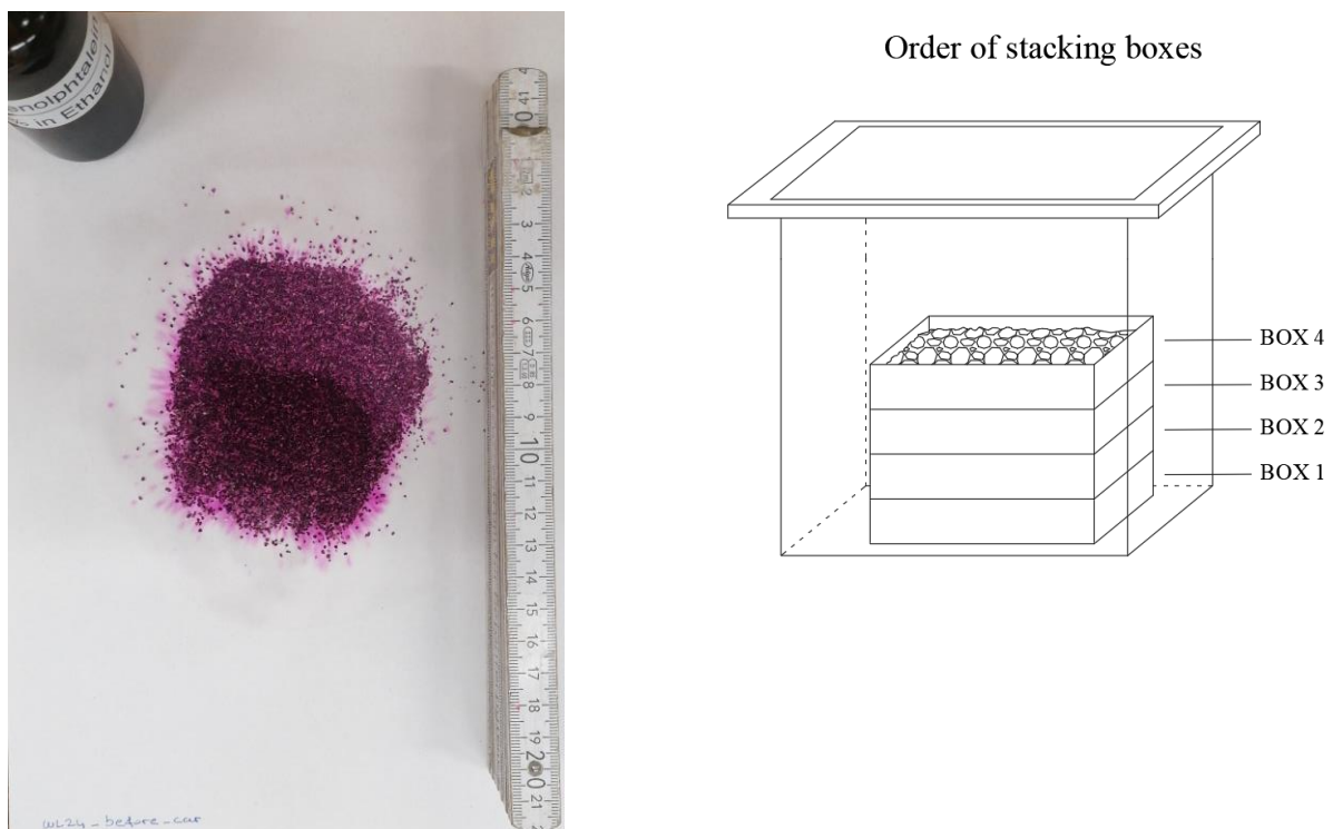
Fig. 31. Phenolphthalein test results before CO 2 curing for experiment WL24.
