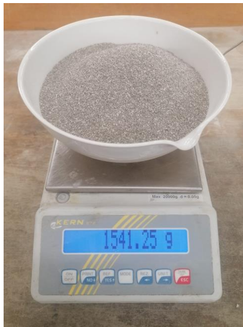
Fig. 33. Mass measurement during moisture content testing
