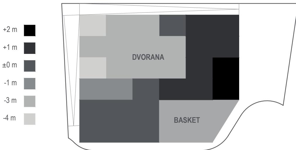
KASKADNO MODELIRANJE TERENA PREMA MODULIMA KONSTRUKTIVNOG RASTERA SHEDA
