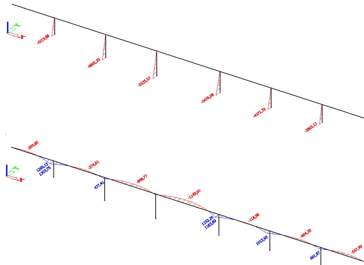
Slika 1.51. -Moment savijanja  $M_z$  (vjetar okomito na prazni most)
