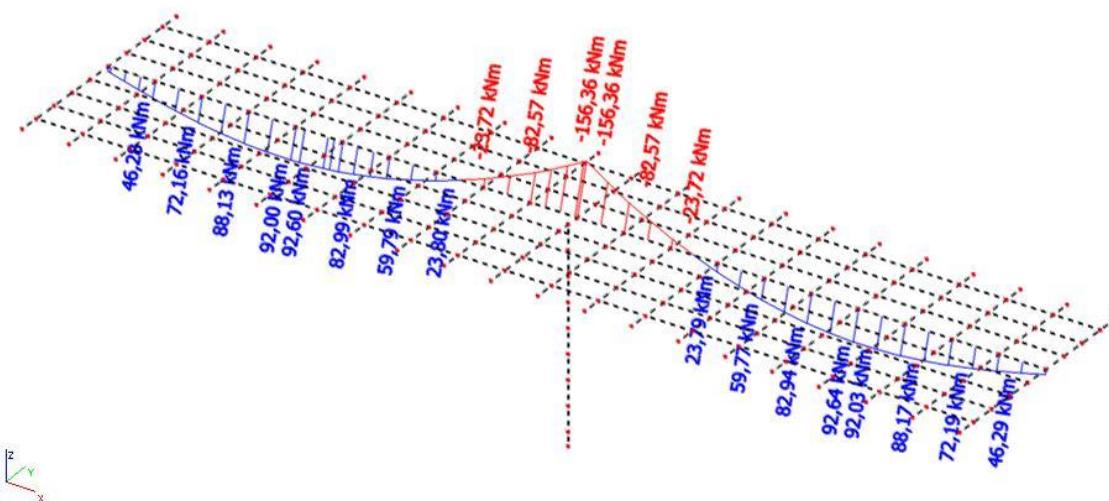
Slika 11: Dodatno stalno - momenti ( $M_y$ ) u kNm
