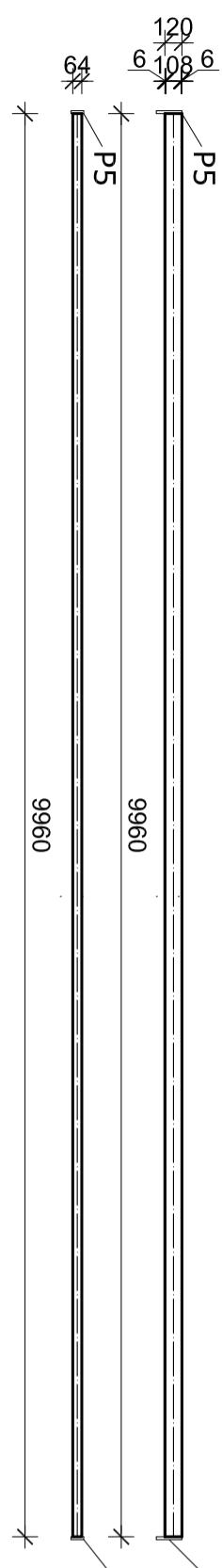
KROVNI SEKUNDARNI NOSAČI (S1-3)  $\perp$  IPE120,  $I=3960$  mm, kom=16
