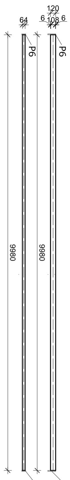
KROVNI SEKUNDARNI NOSAČI (S2-3)  $\perp$  IPE120,  $I=3980$  mm, kom=8
