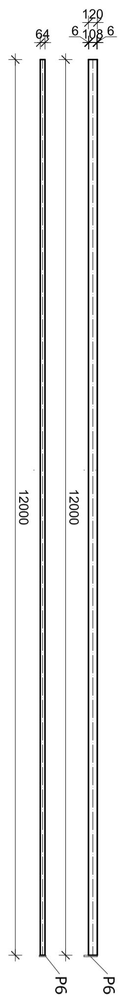
BOČNI SEKUNDARNI NOSAČI (S2-2)  $\perp$  IPE120,  $I=9980$  mm, kom=16
