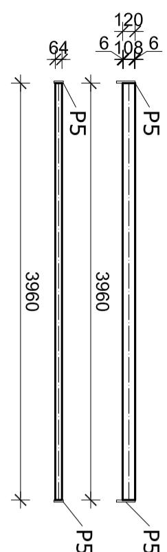
BOČNI SEKUNDARNI NOSAČI (S2-1)  $\perp$  IPE120,  $I=12000$  mm, kom=16
