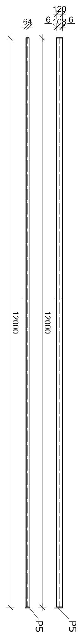
KROVNI SEKUNDARNI NOSAČI (S1-2)  $\perp$  IPE120,  $I=9960$  mm, kom=20
