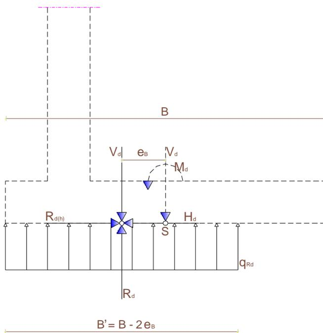
$$V_d = W_u \cdot (1 + k_v) = 1188,71 \cdot (1 + 0,055) = 1254,09 \text{ (kN/ m')} ; x_{\text{krak}} = - 0,33 \text{ (m)}$$
