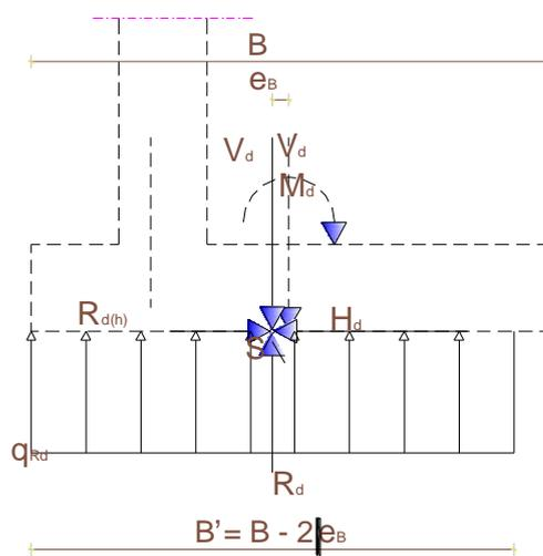
$$V_d = W_u \cdot (1 + k_v) = 434,30 \cdot (1 + 0,055) = 458,19 \text{ (kN/ m')} ; x_{\text{krak}} = - 0,25 \text{ (m)}$$
