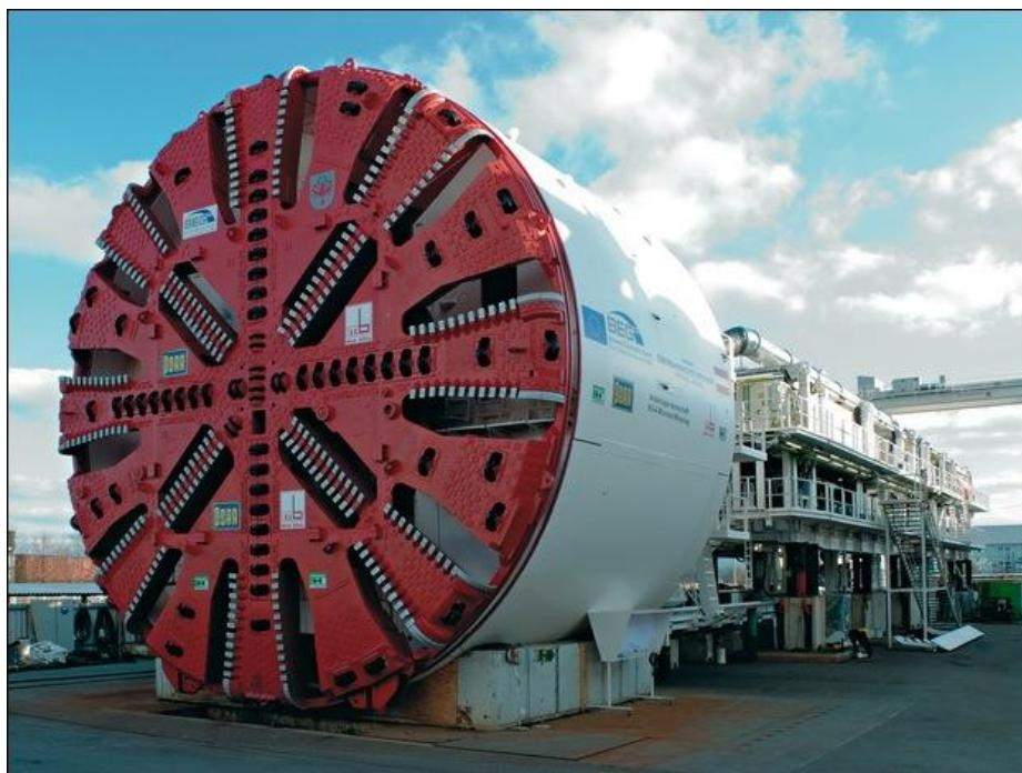
**Slika 3-Herrenknecht TBM [2]**
