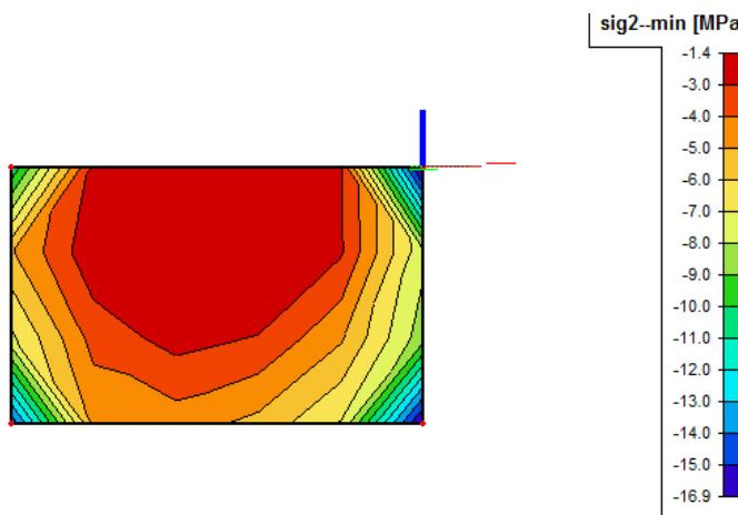
Slika Naprezanja u zidu  $\sigma_c, Rd$ , ANV 10-13
