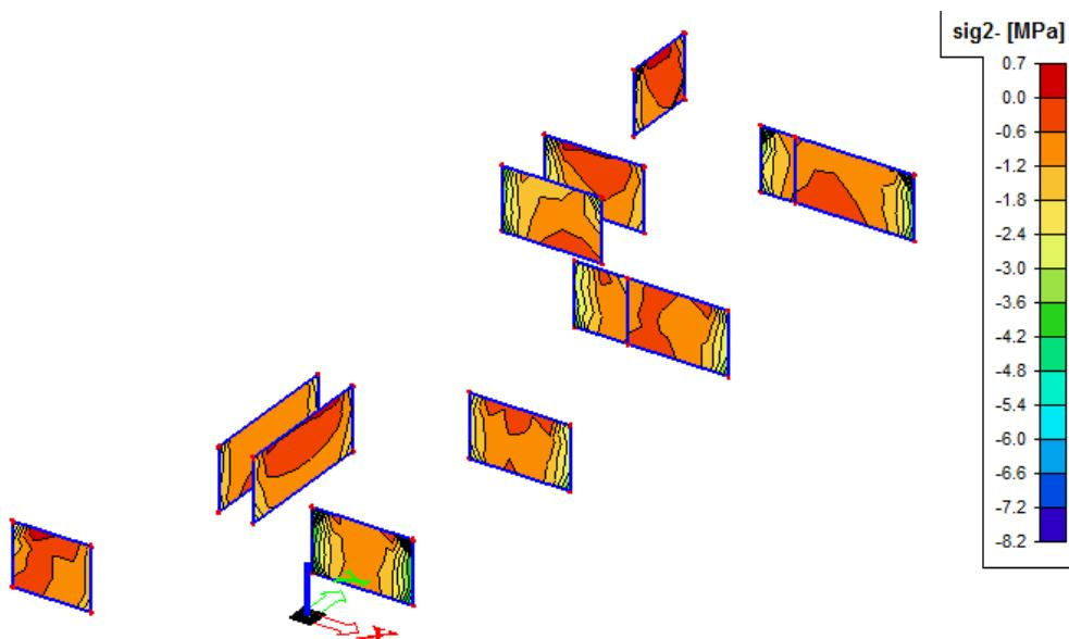
Crtež 7.23. Naprezanja u zidu  $\sigma_c$ , GSU-2:  $1,0*(G_0+G) + 0,3Q$
