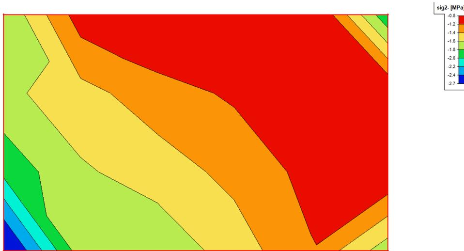
Crtež 8.25. Naprezanja u zidu  $\sigma_{c,GSU-2}: 1,0*(G_0+G) + 0,3Q$
