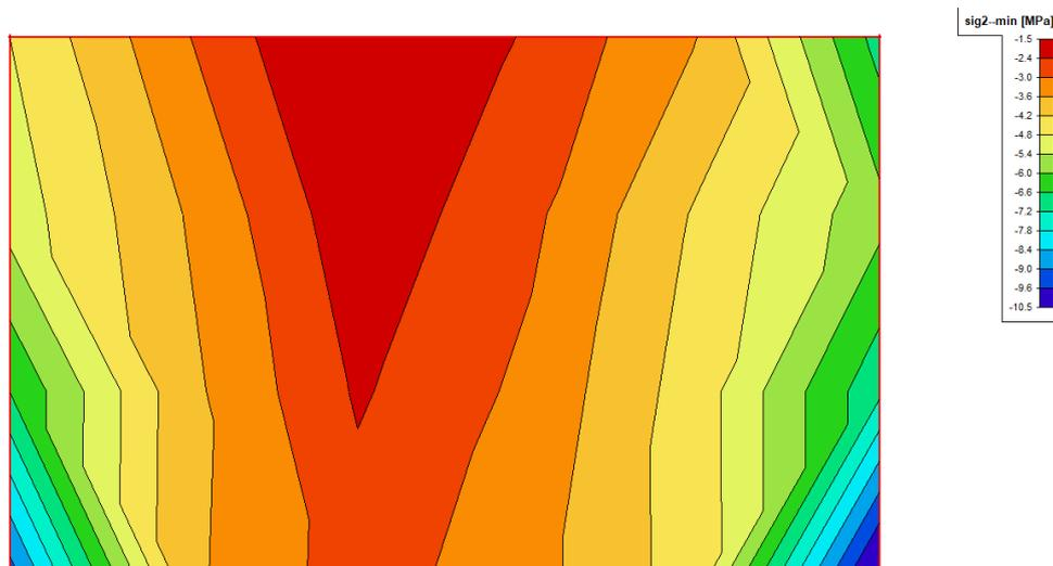
Crtež 8.26. Naprezanja u zidu  $\sigma_{c,Rd}$ , ANV 10-13
