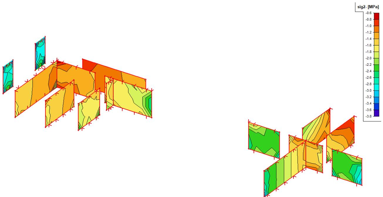
Crtež 8.23. Napreznja u zidu  $\sigma_c$ , GSU-2:  $1,0*(G_0+G) + 0,3Q$
