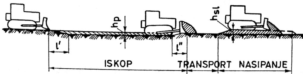
Slika 7: Princip rada buldozera (Izvor: [www.rudar.rgn.hr](http://www.rudar.rgn.hr))
