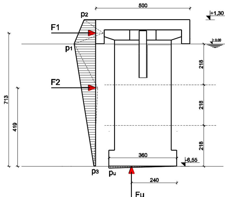
Rezultat proračuna:  $p_1 = 11,4 \text{ kN/m}^2$  ;  $p_2 = 6,2 \text{ kN/m}^2$  ;  $p_3 = 1,0 \text{ kN/m}^2$  ;  $p_u = 1,0 \text{ kN/m}^2$
