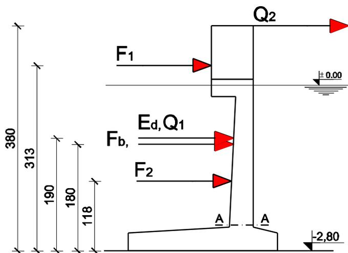
Stalna opterećenja .....  $F_1 = 2,0 \text{ kN/m}$  ,  $F_2 = 21,0 \text{ kN/m}$
