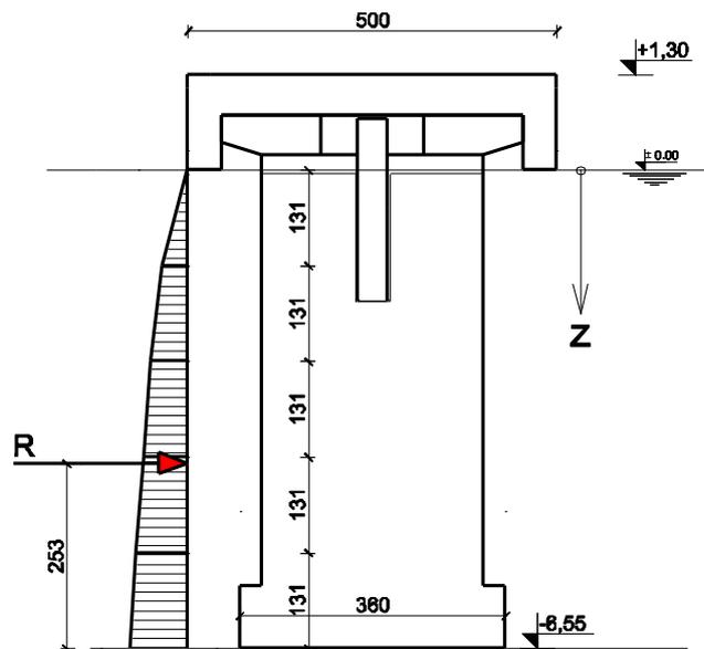
Sila kojom voda djeluje na stup:  $R_s = 33,0 \text{ kN/m}' \cdot 3,0\text{m}' = 99,0 \text{ kN}$
