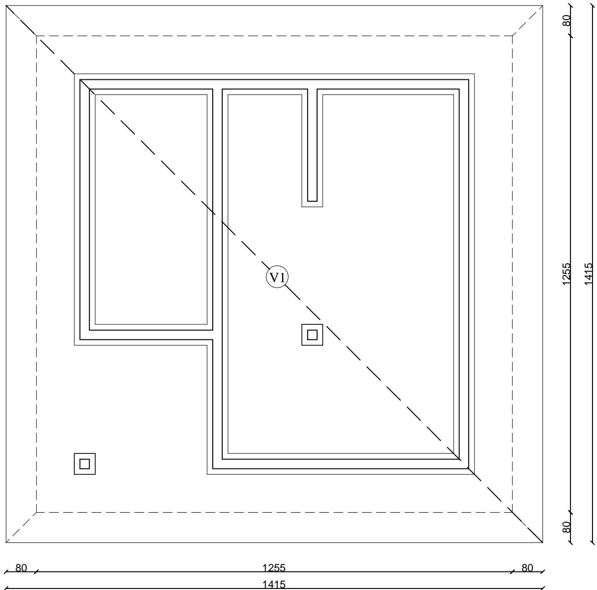
$$\text{Volumen krnje piramide} = \frac{1}{3} \times h (B_1 + B_2 + \sqrt{(B_1 \times B_2)})$$
