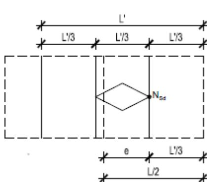
$$\begin{aligned} \sigma_{ekv} &= \frac{2 * (G + N_{SD})}{L' * B} \\ &= \frac{2 * (234,38 - 7,73)}{0,69 * 2,5} \\ &= 262,78 \text{ kN/m}^2 \\ &< \sigma_{tla,lim} \\ &= 300 \text{ kN/m}^2 \end{aligned}$$
