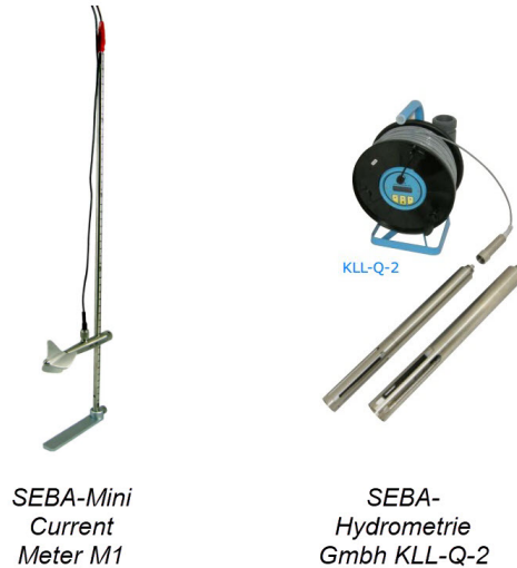
FIGURE 4.6: Hydrometric wing (left) and salinity probe (right).
