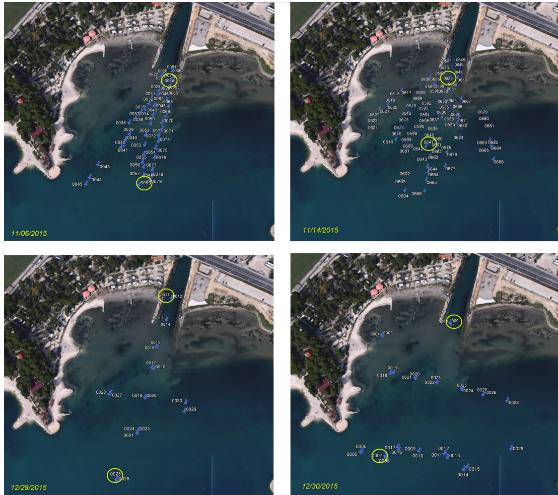
FIGURE 4.10: Recorded positions for different salinity measurement campaigns with indicated dates and points represented in the results.
