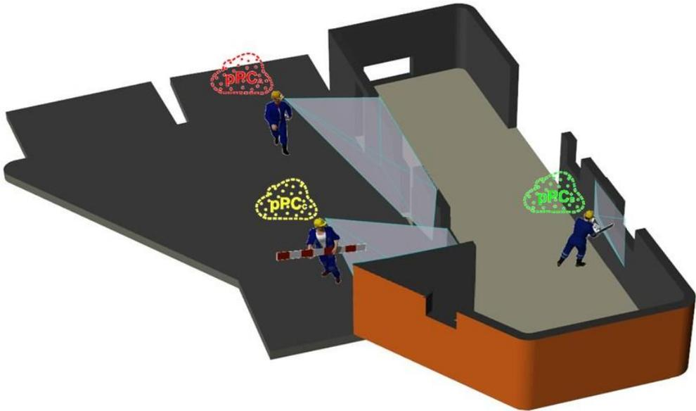
**Figure 4.3.** A scenario of indoor and outdoor continuous partial point cloud acquisition on-site using multiple helmet-mounted scanners [8]
